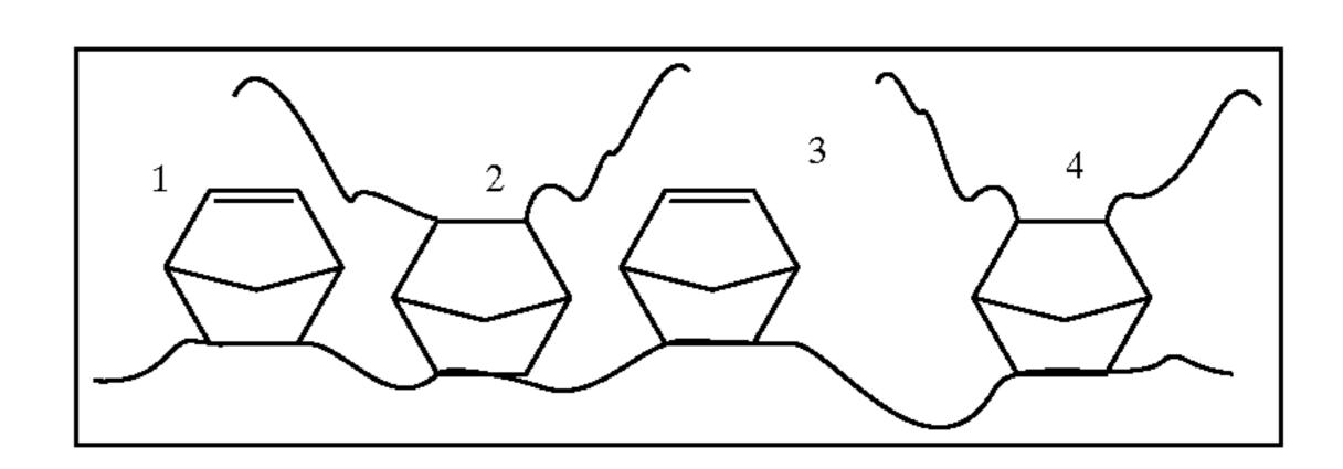
Stabilization of that residual unsaturation provides preferred structures for subsequent cross-linking (e.g., by a wire or cabling manufacturer) such that less cross-linking agent, such as an organic peroxide, needs to be used relative to cross-linking of a polymer with less residual unsaturation. 4-arm star LCB or similar moieties provide enhanced rheological behavior that will lead to easier extrusion and superior melt strength relative to polymers without those structures.
