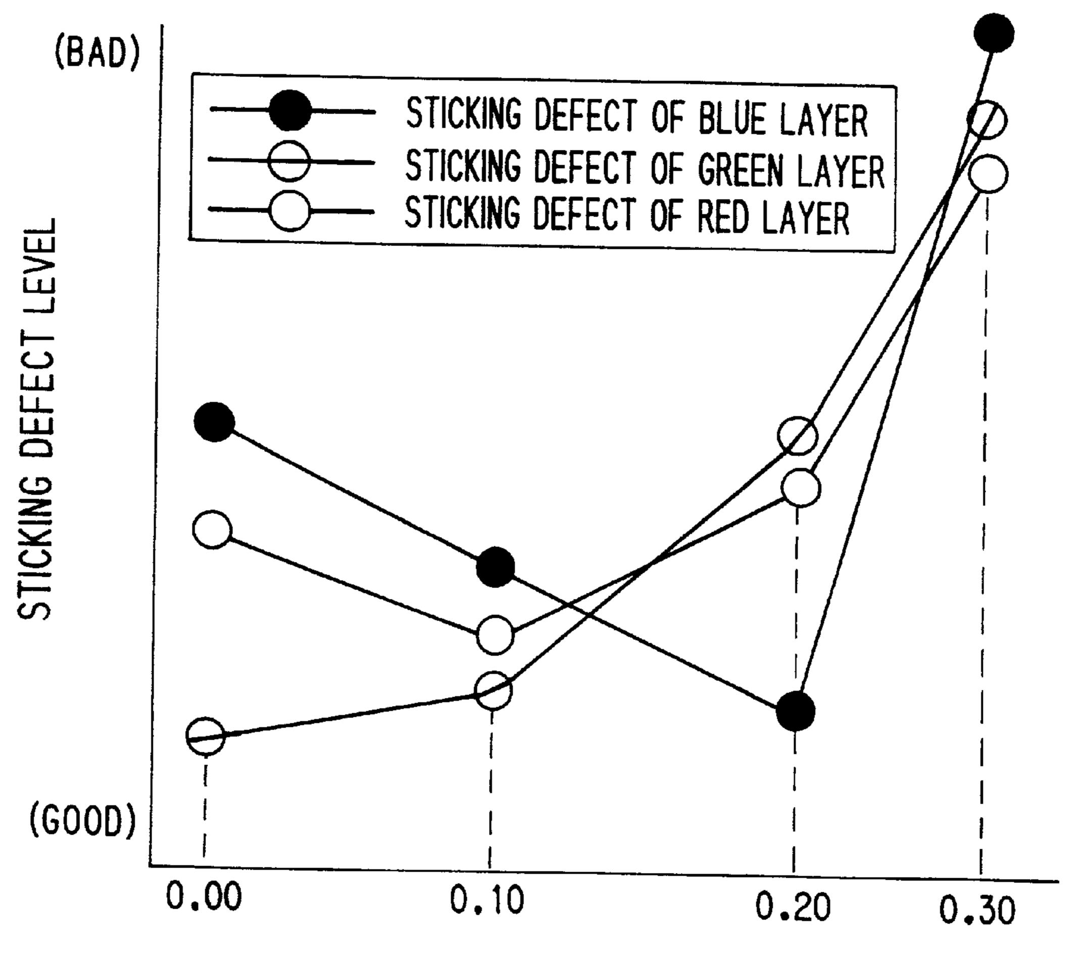
CORRECTION AMOUNT OF CENTRAL VALUE OF DRAIN VOLTAGE (V)
