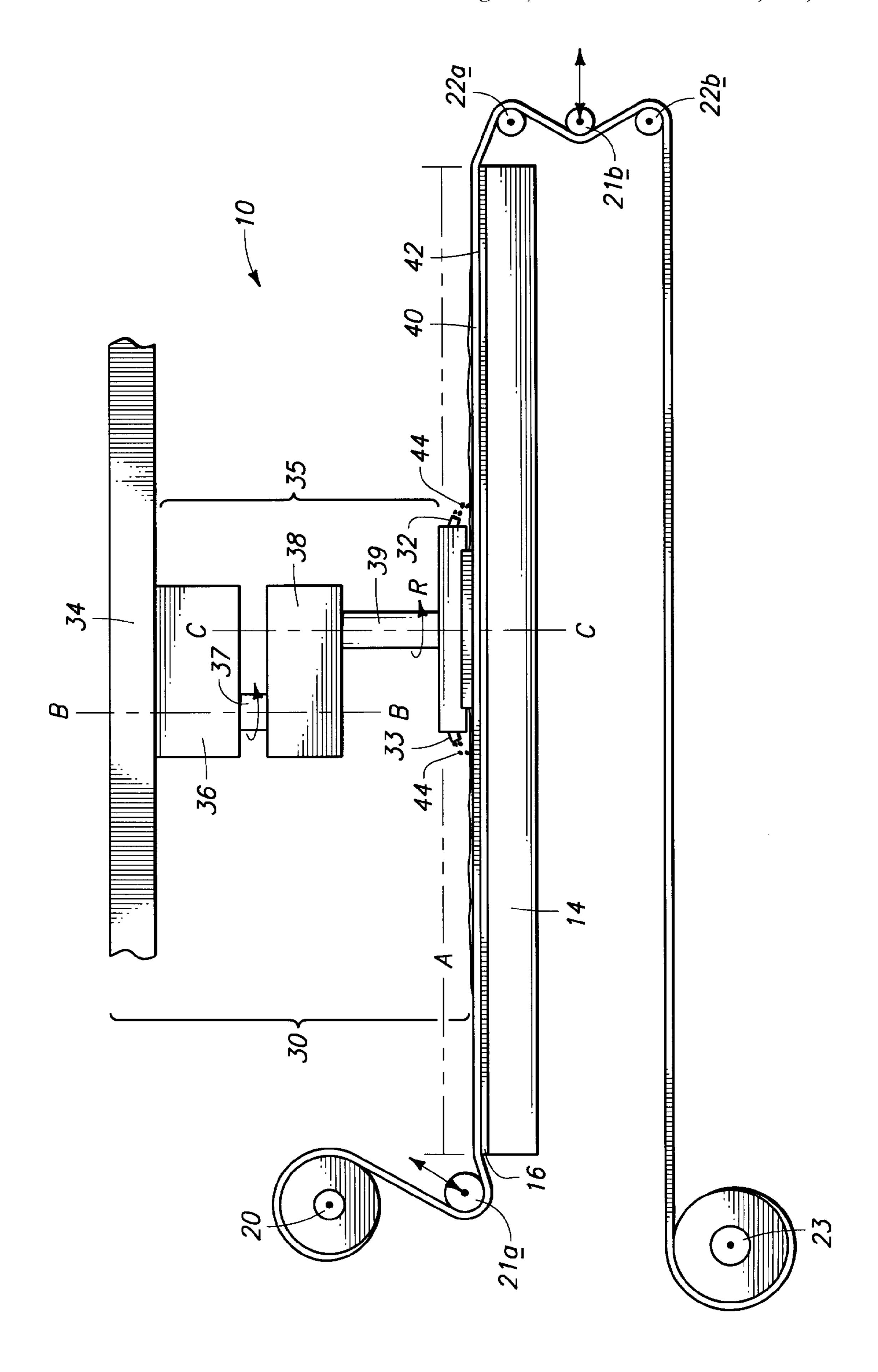
TUNGSTEN CHEMICAL-MECHANICAL POLISHING PROCESS USING A FIXED ABRASIVE POLISHING PAD AND A TUNGSTEN LAYER CHEMICAL-MECHANICAL POLISHING SOLUTION SPECIFICALLY ADAPTED FOR CHEMICAL-MECHANICAL POLISHING WITH A FIXED ABRASIVE PAD
