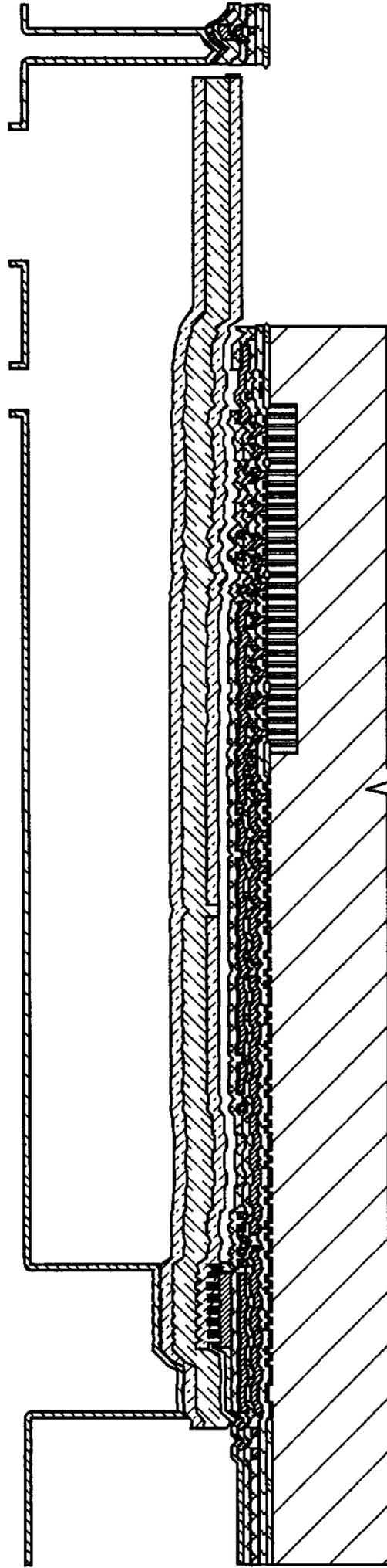
Detach from wafer blank, etch sacrificial material
