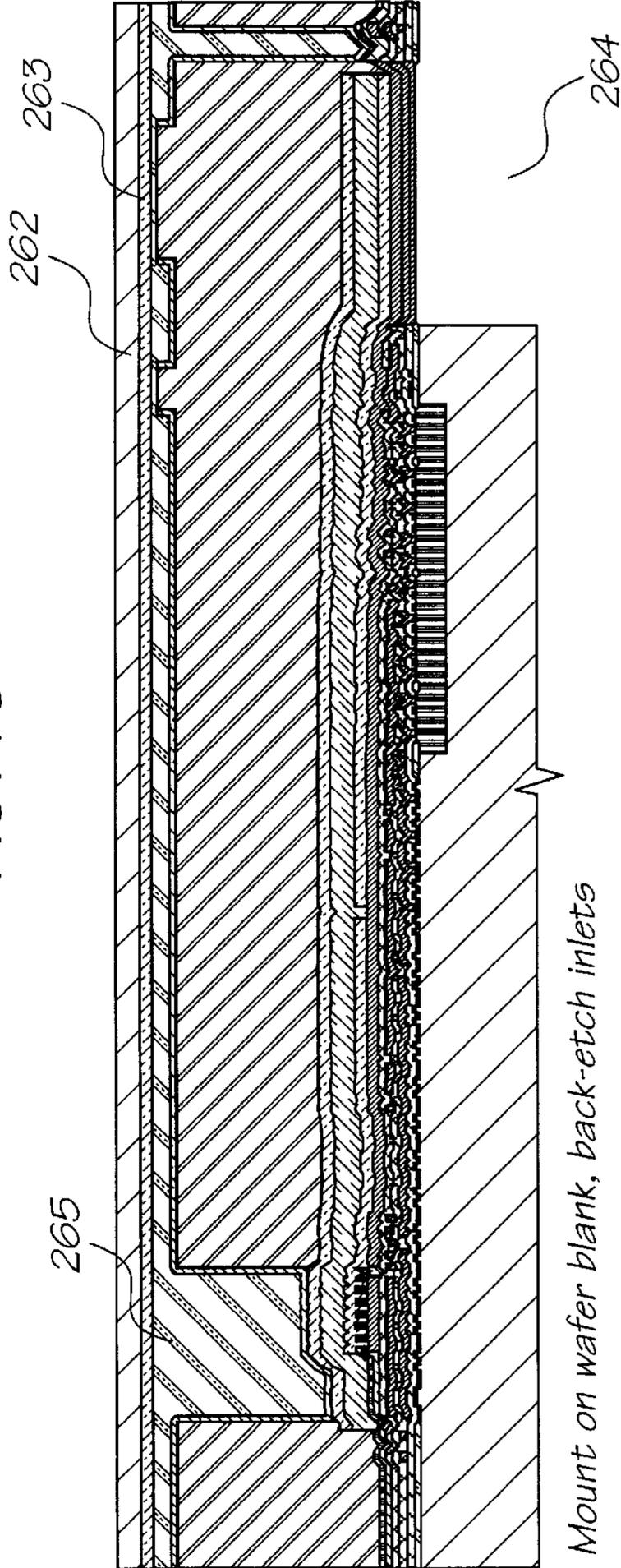
Mount on wafer blank, back-etch inlets
