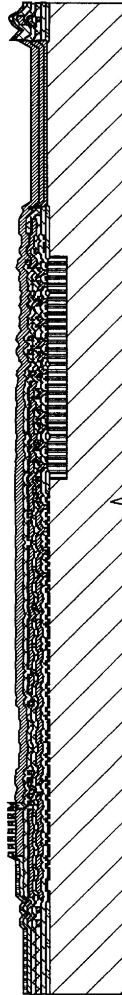
Deposit passivation oxide & nitride, etch vias
