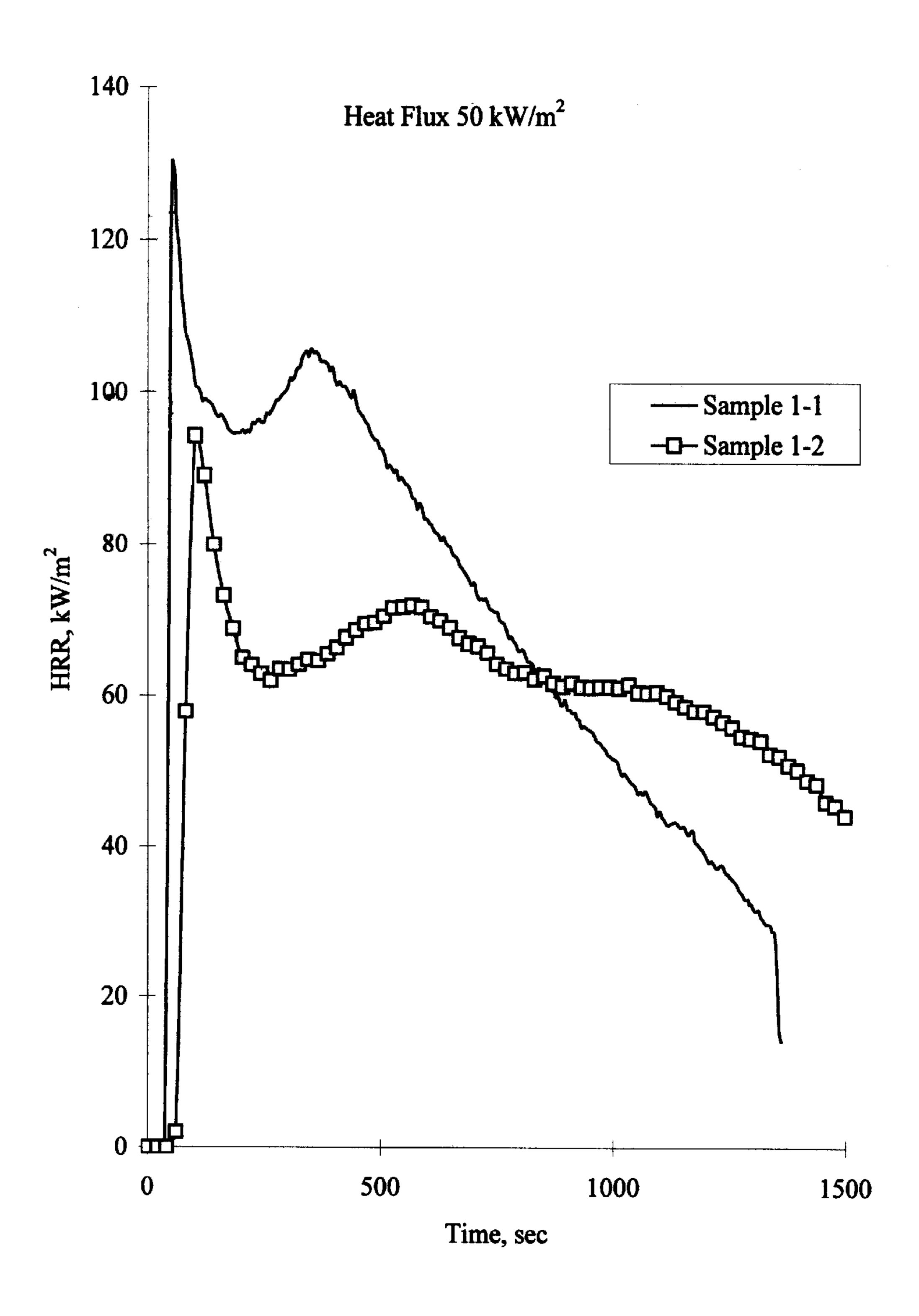
Figure 1. The HRR as a Function of Time for Model Elastomers.
