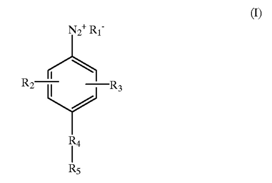
wherein  $R_1$  is an anion,  $R_2$  and  $R_3$  represent optional substitution,  $R_4$  is —N— or —S— and  $R_5$  is a group which, after exposure of the plate, renders the residue of the diazo salt oleophilic and fount solution insoluble.
