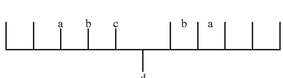
The methyl groups labeled "a", "b", "c", and "d" give the most intense signals in the C-13 NMR spectra. The intensity of the peak represent by "d" is a direct measure of the 10 number of mistakes (mrrm) in monomer  $\pi$ -face selectivity (re vs. si), providing the probability of "errors" in close succession is negligible. The C-13 NMR pentad intensities for polymer produced with rac-Me<sub>2</sub>Si[2-MeInd]<sub>2</sub>ZrCl<sub>2</sub> at 60° C. is given below:
