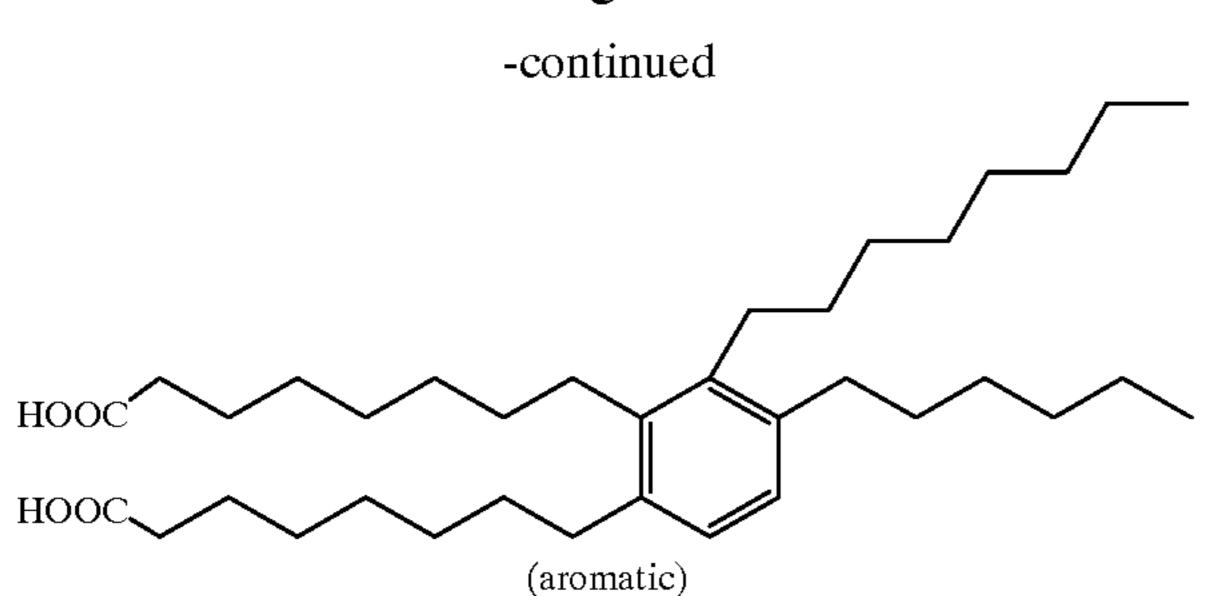
Structures for components of trimer acids are similar to those of dimer acids except that they contain an additional carboxylic acid group terminating from another hydrocar- 15 bon chain, they contain an additional non-functional hydrocarbon chain, and they contain a greater portion of bicyclic compounds.
