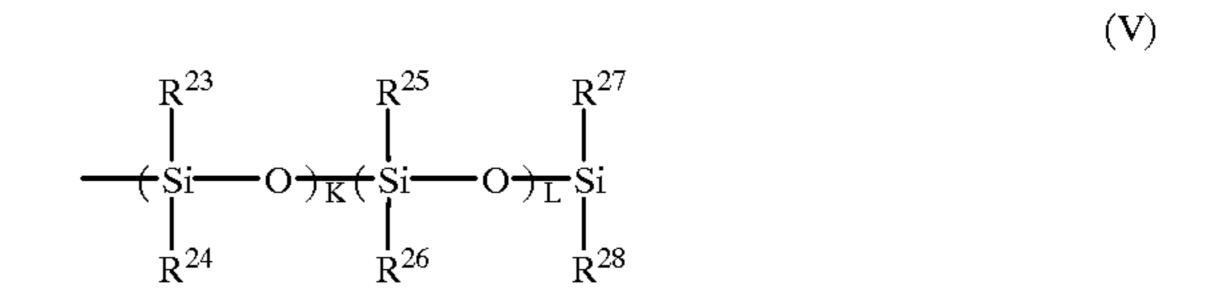
in which each of R<sup>23</sup>, R<sup>24</sup>, R<sup>25</sup>, R<sup>26</sup>, R<sup>27</sup> and R<sup>28</sup> is independently an alkyl group having 1 to 3 carbon atoms or phenyl group, K is an integer of 1 to 1500, L is 0 or an integer of 1 to 1500, and (K+L) is an integer of 1 to 1500;
