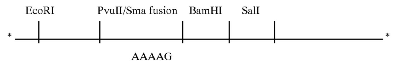
(c) pCOWT1 is cut with SalI, blunt-ended with T4 DNA polymerase, and EcoRI linkers are added followed by digestion wit EcoRI to produce fragment 12 (0.6 kb).
