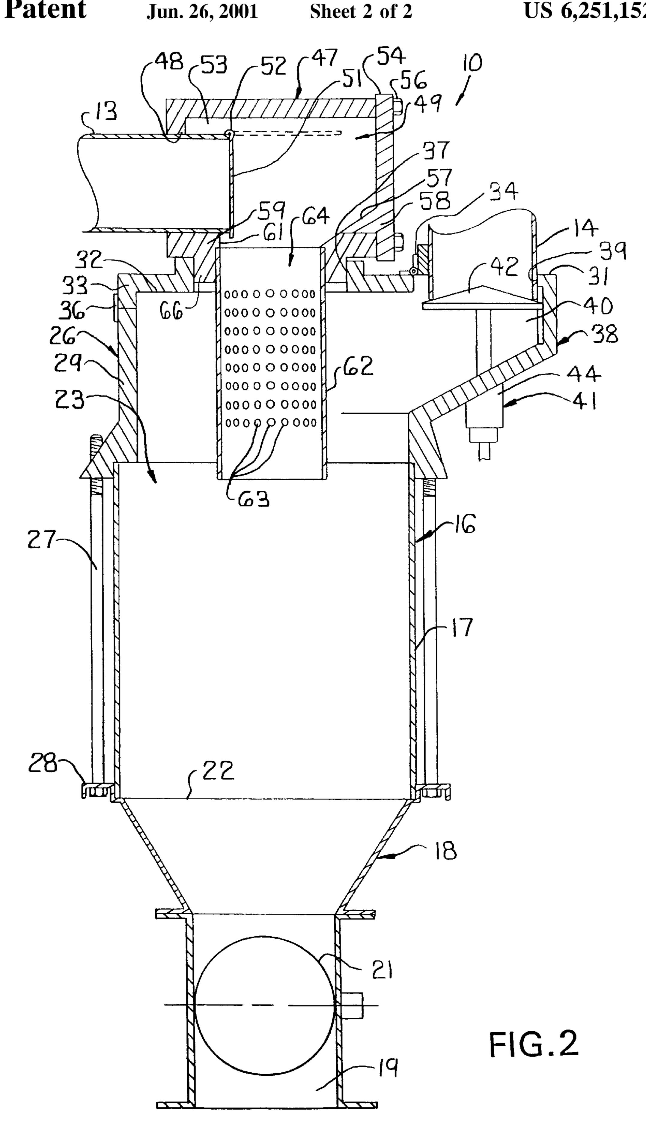
VACUUM RECEIVER FOR SEPARATING PARTICLES IN A GAS FLOW HAVING AN INLET HOUSING INSERTABLE AND REMOVABLE FROM AN OPENING IN A COVER OF THE VACUUM RECEIVER
