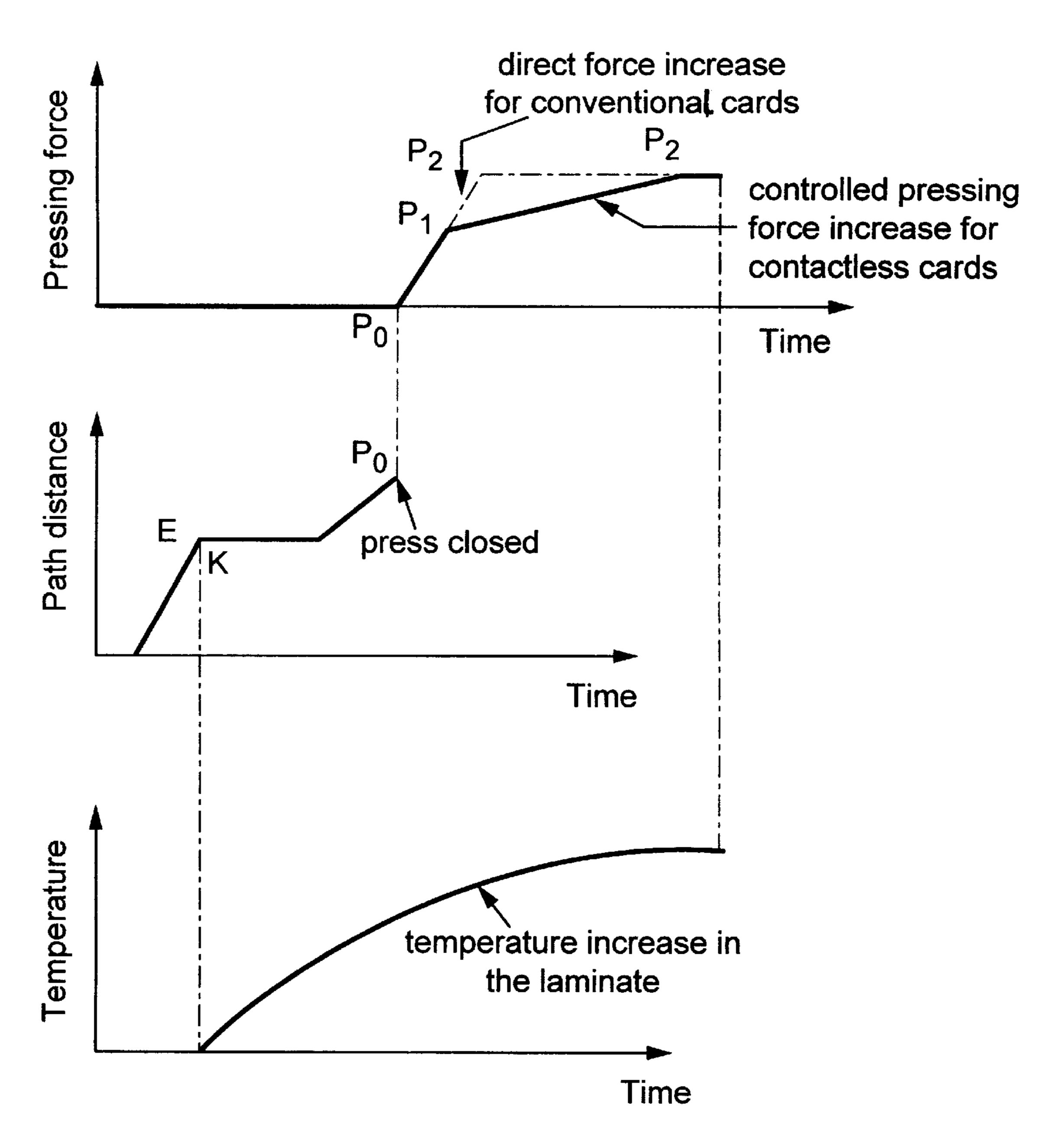
E = sensor for switching off the closing path after placement on the uppermost heating plate
