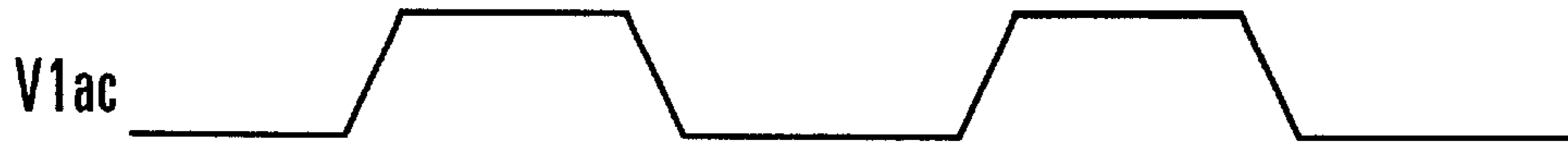
FIG.21A BOTH V_{1ac} AND V_{2ac} ARE TRAPEZOIDAL WAVEFORMS
