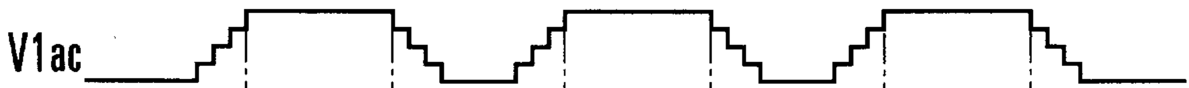
FIG.21G BOTH V_{1ac} AND V_{2ac} ARE STAIRCASE WAVEFORMS FORMED BY POWER SUPPLY CIRCUIT 10B
