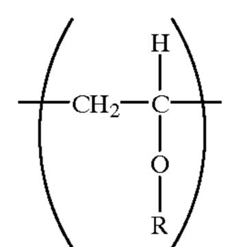
where R is an organic substituent, wherein the polyvinyl alcohol moiety has a hydroxyl content that ranges from 0% to about 5% by weight when —OR is an acetate.
