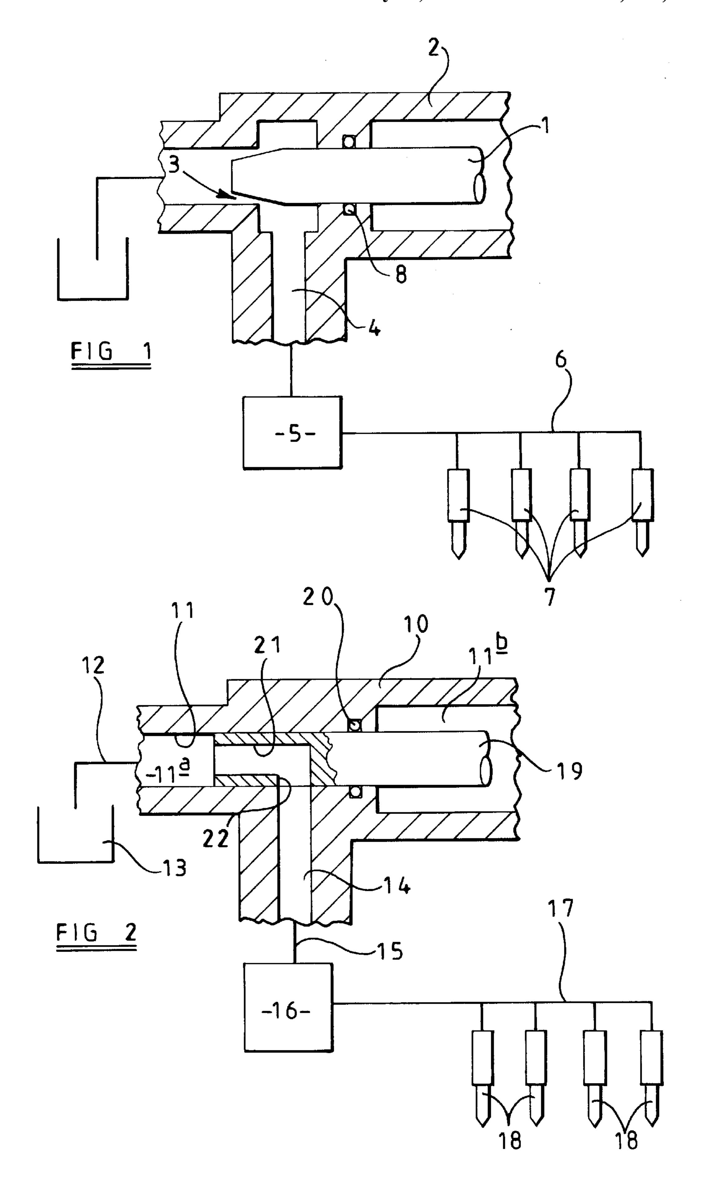
This invention relates to a fuel system for use in supplying a fuel of the type which is viscous at relatively low temperatures to a combustion space of an associated internal combustion engine of the compression ignition type. The invention is particularly applicable to a fuel system of the common rail type.
