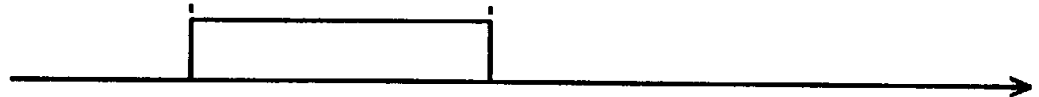
FIG. 3 c WELDING START SIGNAL
