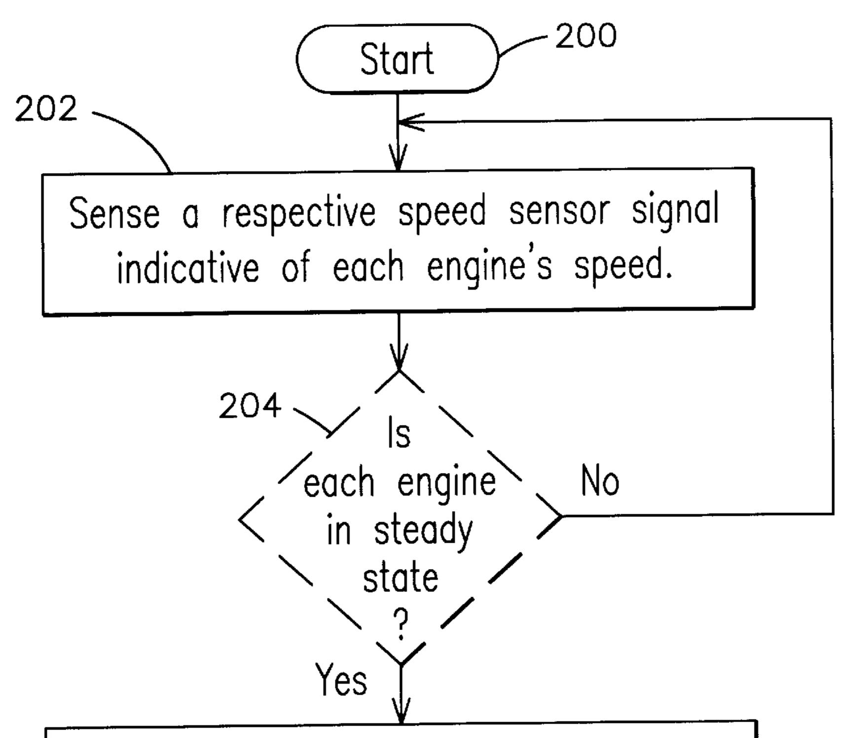
Compare each speed sensor signal relative to one another to supply a signal based on the magnitude of engine speed differences.
