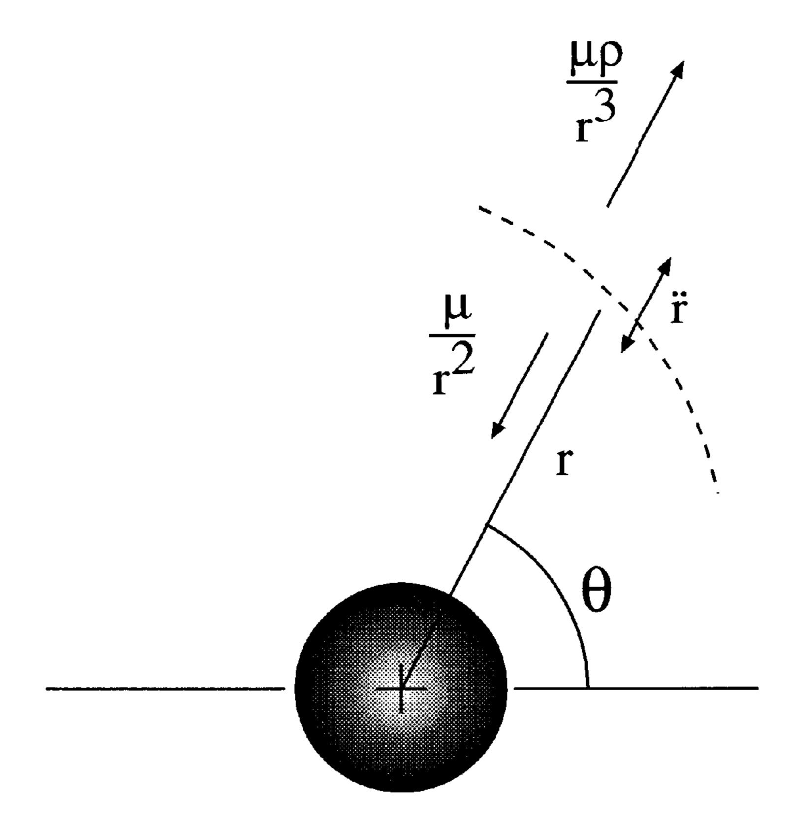
*FIG. 5*Two-Body Polar Coordinate System
