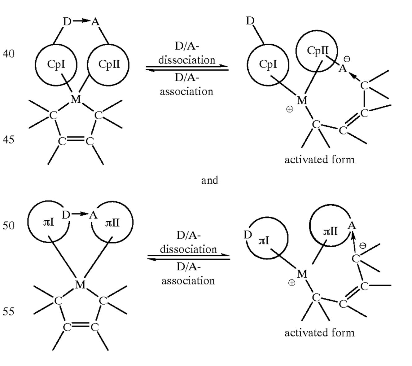
The bonding site between the transition metal M and H or substituted or unsubstituted C, in the formula example the still bonded substituted C of the butadienediyl dianion shown, is then the site for the olefin insertion for the polymerization.
