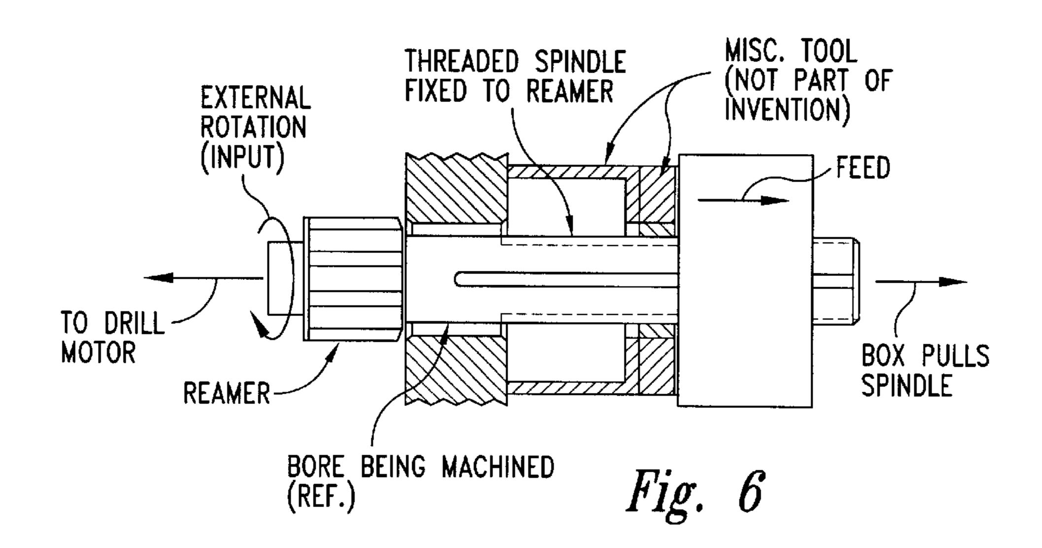
OUTPUT GEAR 4 ROTATES AT A SPEED SLIGHTLY LESS (90%) THAN INPUT GEAR 3. THIS ALLOWS FOR A MICRO-FEED (PULL) OF THREADED SPINDLE 6 WHICH IS DIRECTLY COUPLED TO CUTTER
