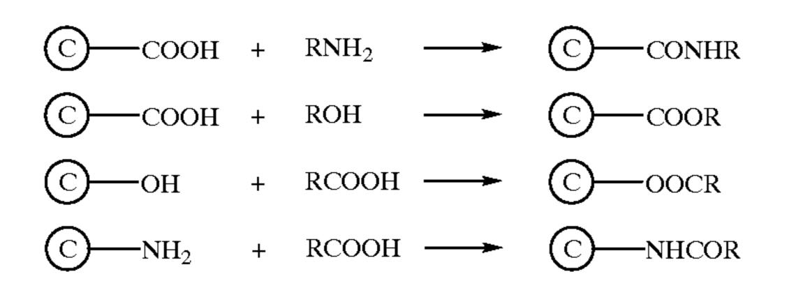
The novelty of this process resides in the fact that the reaction is carried out in such a manner that the carbon which is intended to be modified by polymer segments is in suspension in a solution containing the polymer which is intended to be grafted, and in the fact that the solvent is selected so as to be able to carry out the reaction of dehydration between a carboxyl function and an amine and/or an hydroxyl function at a suitable temperature.
