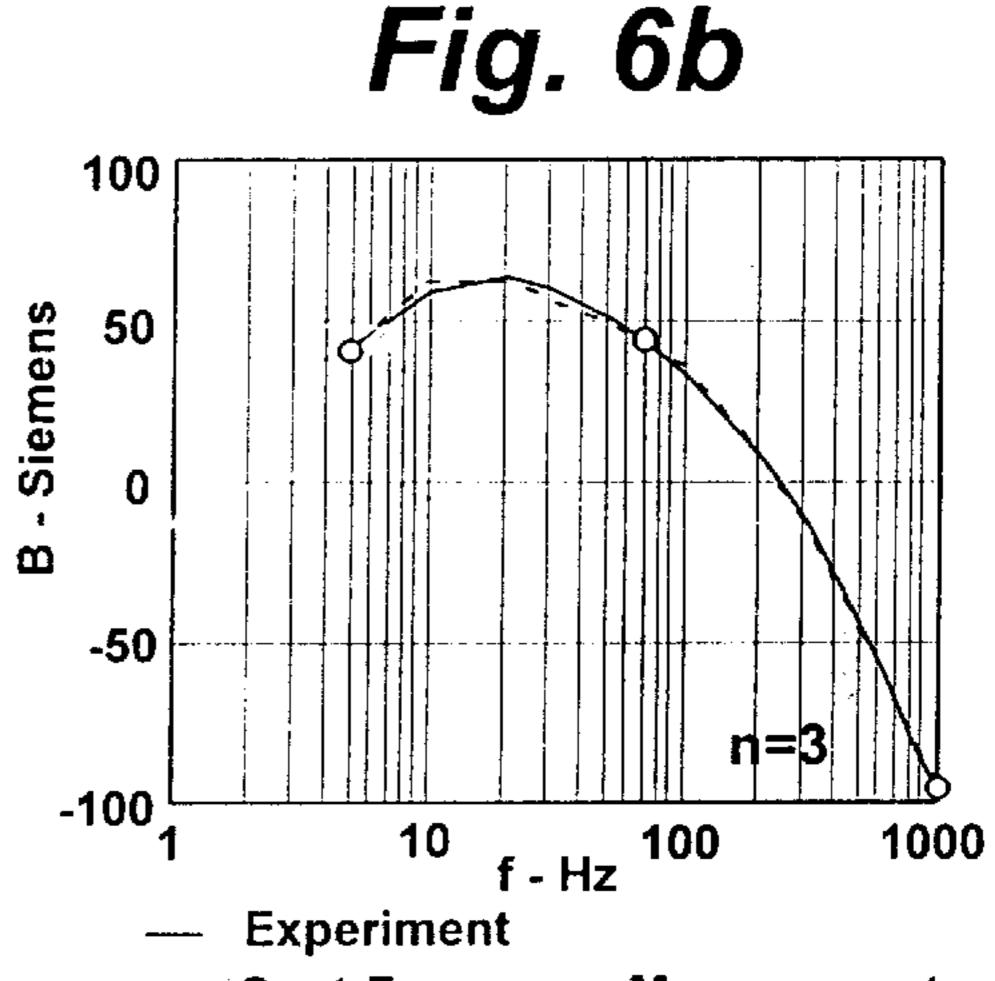
oo Spot-Frequency Measurements - - Calculated from Fig. 5 Model
