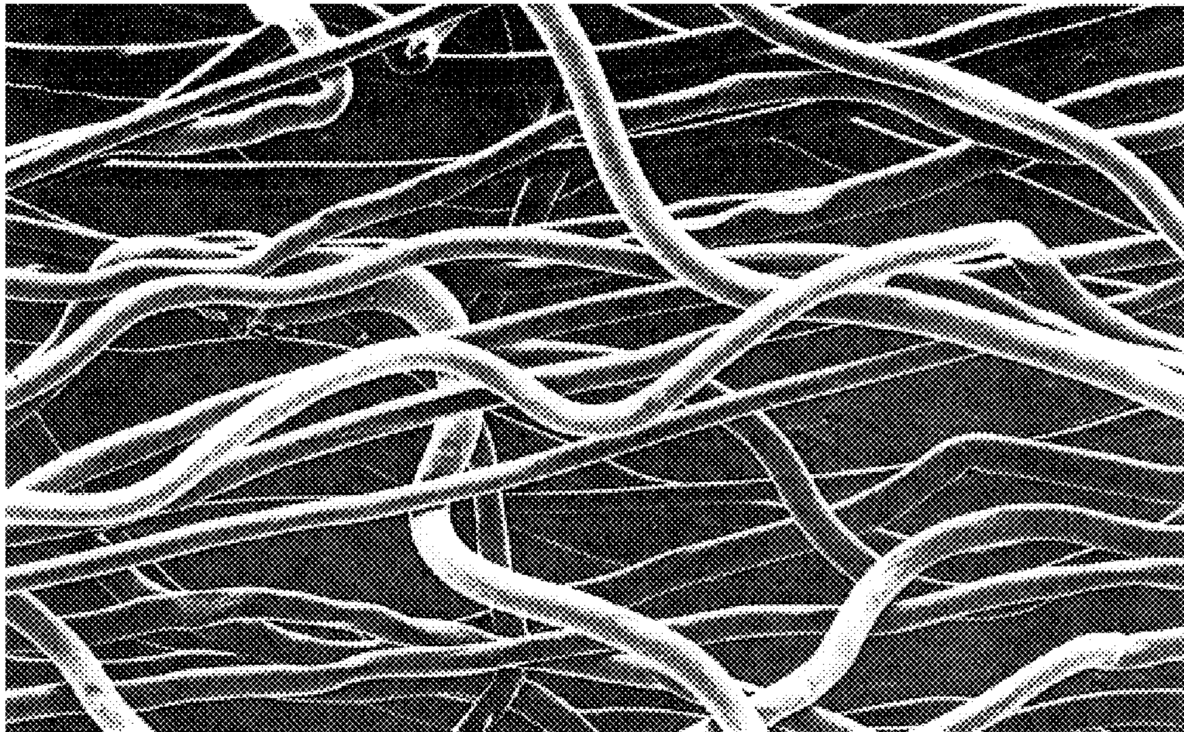
Melt Blown Fiber - 100X
