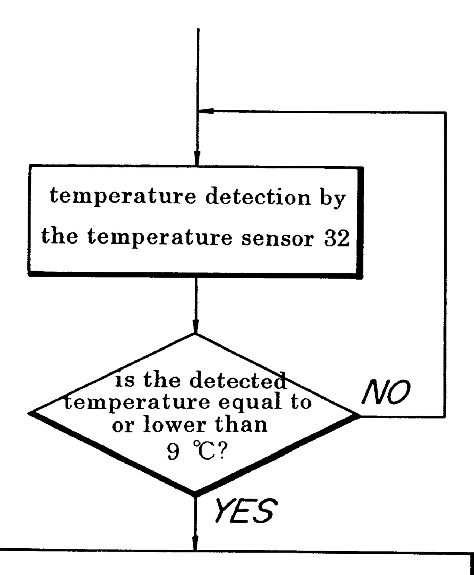
close the cooling/heating switch valve 11 close the flow control valve 9 stop the electric pump 8
