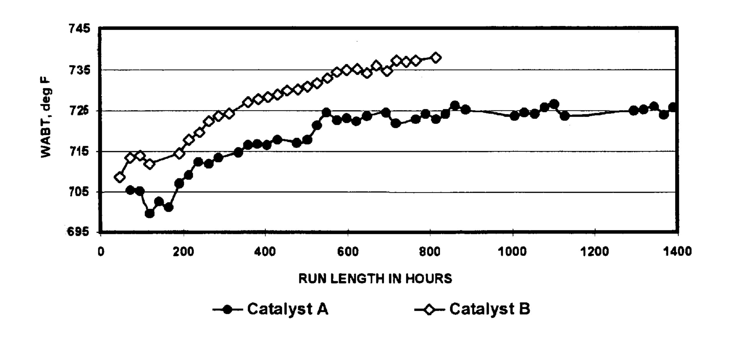
FIGURE 2. WABT REQUIRED FOR 88% SULFUR REMOVAL
