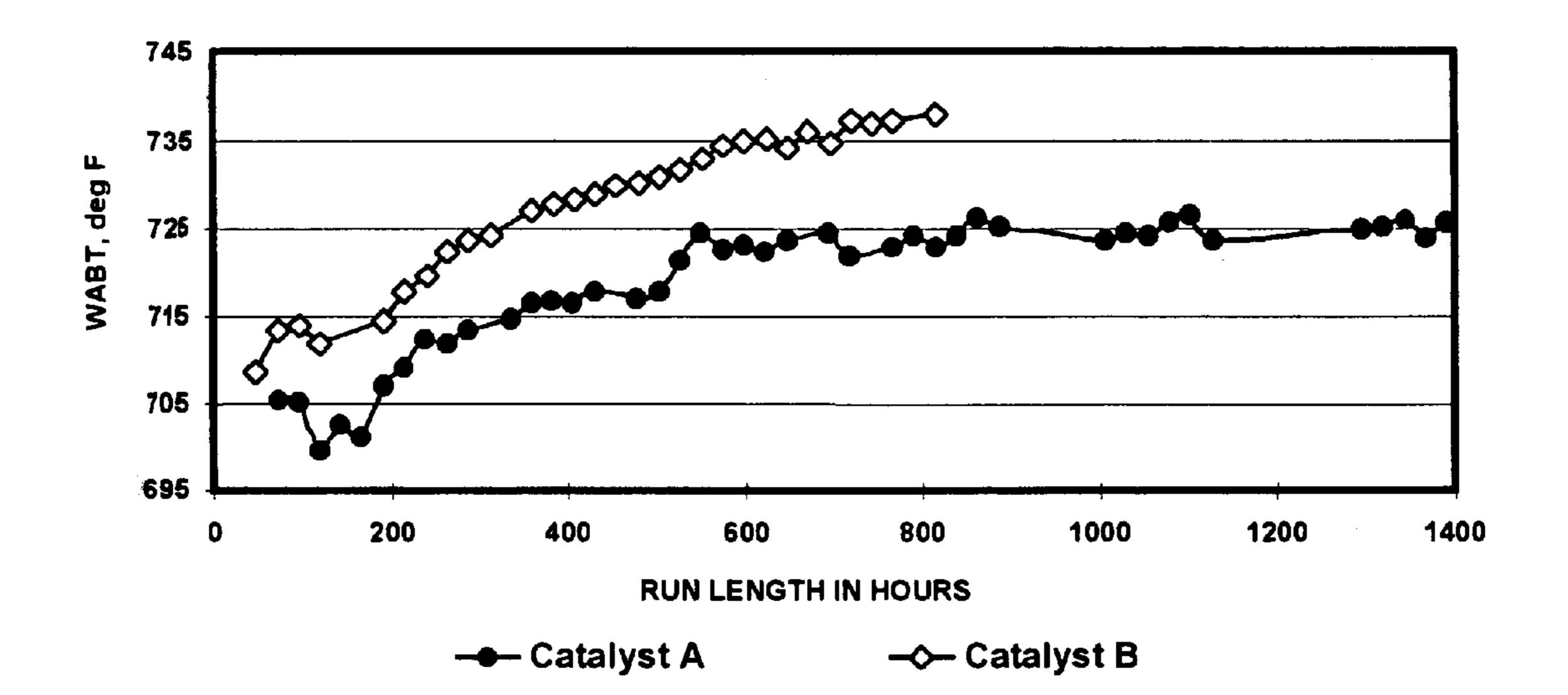
FIGURE 1. WABT REQUIRED FOR 88% SULFUR REMOVAL
