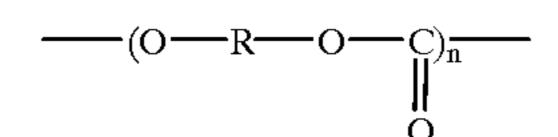
wherein R represents a straight chain or branched hydrocarbon group having from 2 to 20 carbon atoms, a pressure-sensitive adhesive sheet, a sealing material, a reinforcing sheet, and a pressure-sensitive sheet for printing, each having the pressure-sensitive adhesive composition.
