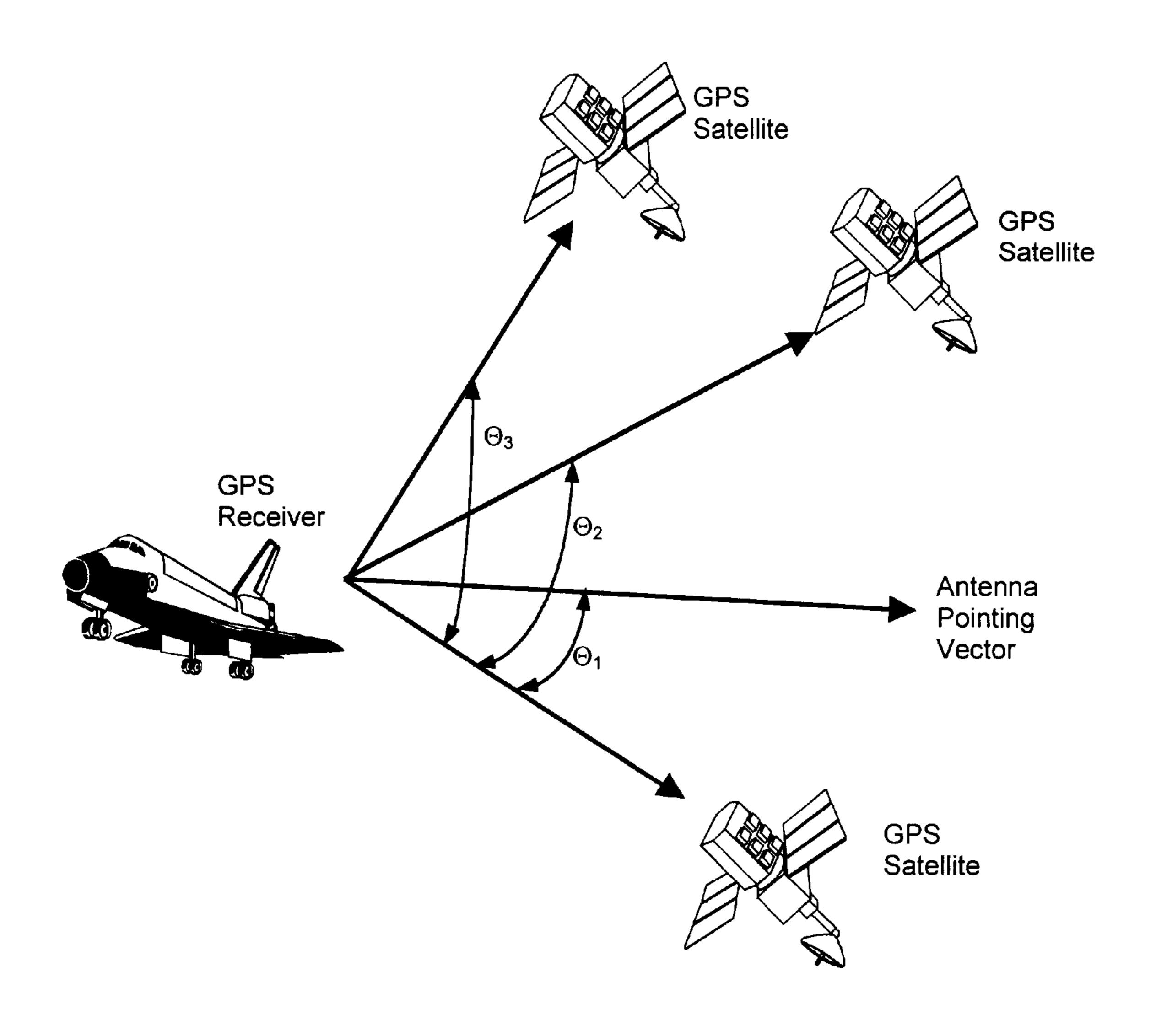
Θ<sub>1</sub> is the smallest angle between the APV and a GPS satellite
