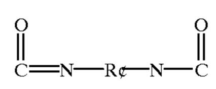
where R' is a C<sub>2</sub> to C<sub>12</sub>, a cycloalkyl or cycloalkyl-containing group, an aryl or aryl-containing group, 4,4'-diphenylmethane, toluene, naphthalene, 4,4'-dicyclohexylmethane, cyclohexyl, 3,3'-dimethylphenyl, 3,3'-dimethyl-diphenylmethane, 4,6'-xylylene, 3,5,5-trimethylcyclohexyl, 2,2,4-trimethylhexamethylene or p-phenylene.
