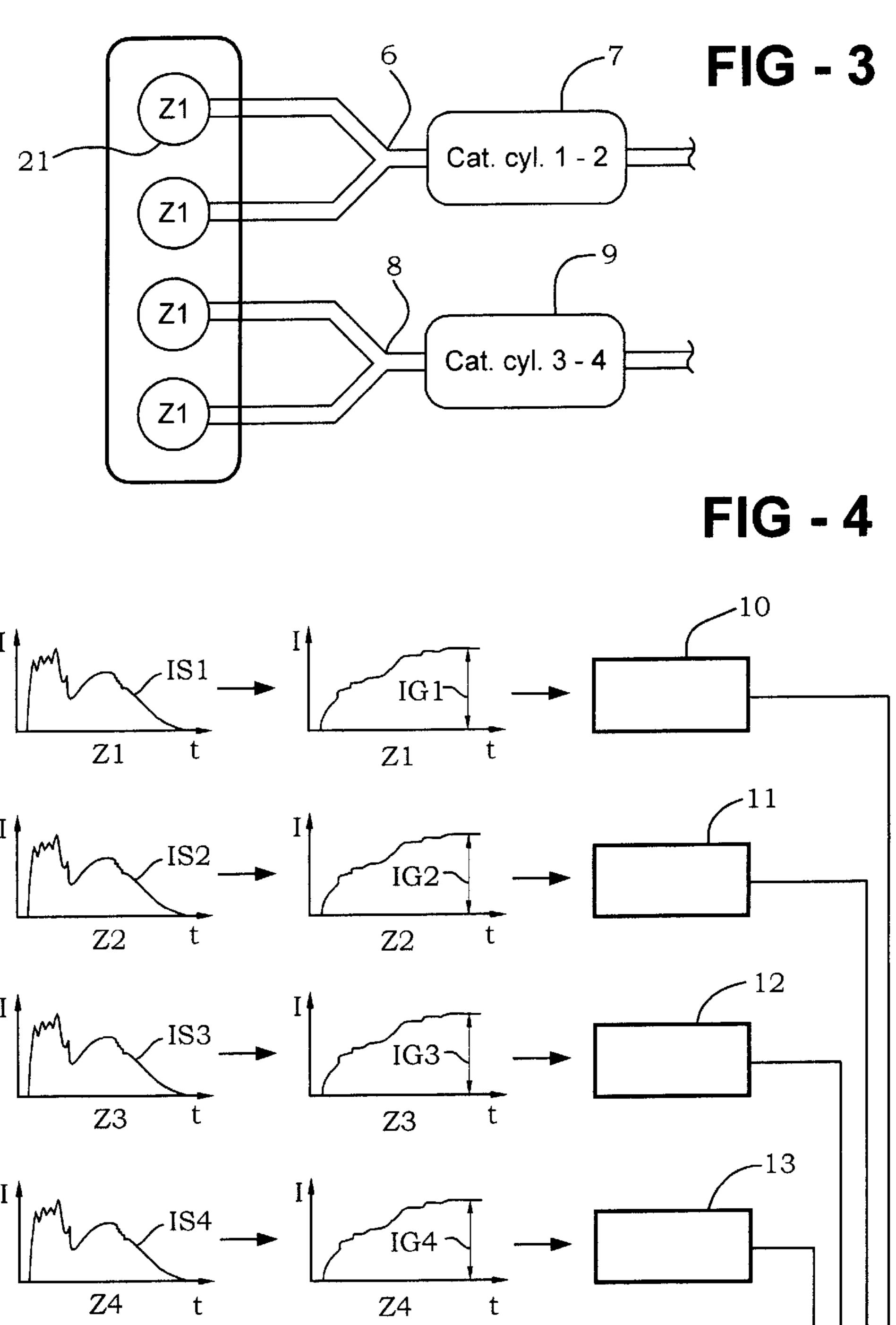
If average ion current of cyl. 1 - 2 higher than average ion current of cyl 3 - 4 cat. of cyl. 3 - 4 may be defective
