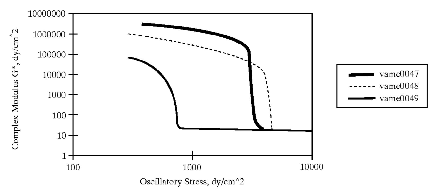
The elastic modulus G' is a measure of a materials ability to store recoverable energy. This energy storage can be the result of the ability of a complex polymer, structural network, or a combination of these to recover stored energy 45 after a deformation. The loss modulus G" is a measure of the unrecoverable energy which has been lost due to viscous dampening.
