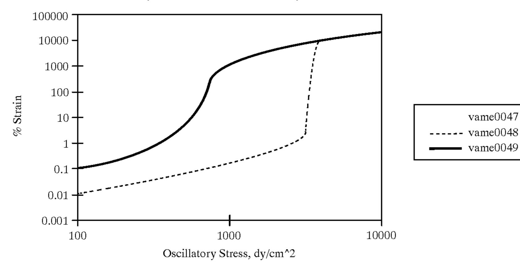
The above plot shows that there is a sharp transition into the flow regime for Composition D at 2750 dy/cm<sup>2</sup> (about 7% strain) and Composition E at 3700 dy/cm<sup>2</sup> (about 10%) strain). Composition F shows a much more gradual transition into flow. The transition into the flow regime for 25 Composition F begins at approximately 300 dynes/cm<sup>2</sup> (about 1% strain).
