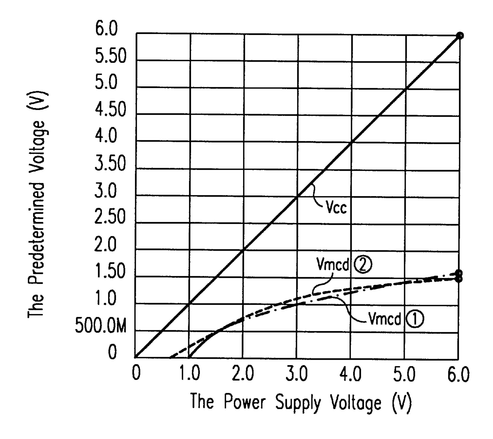
Vmcd ①: Vmcd of the Conventional Constant Voltage Circuit
