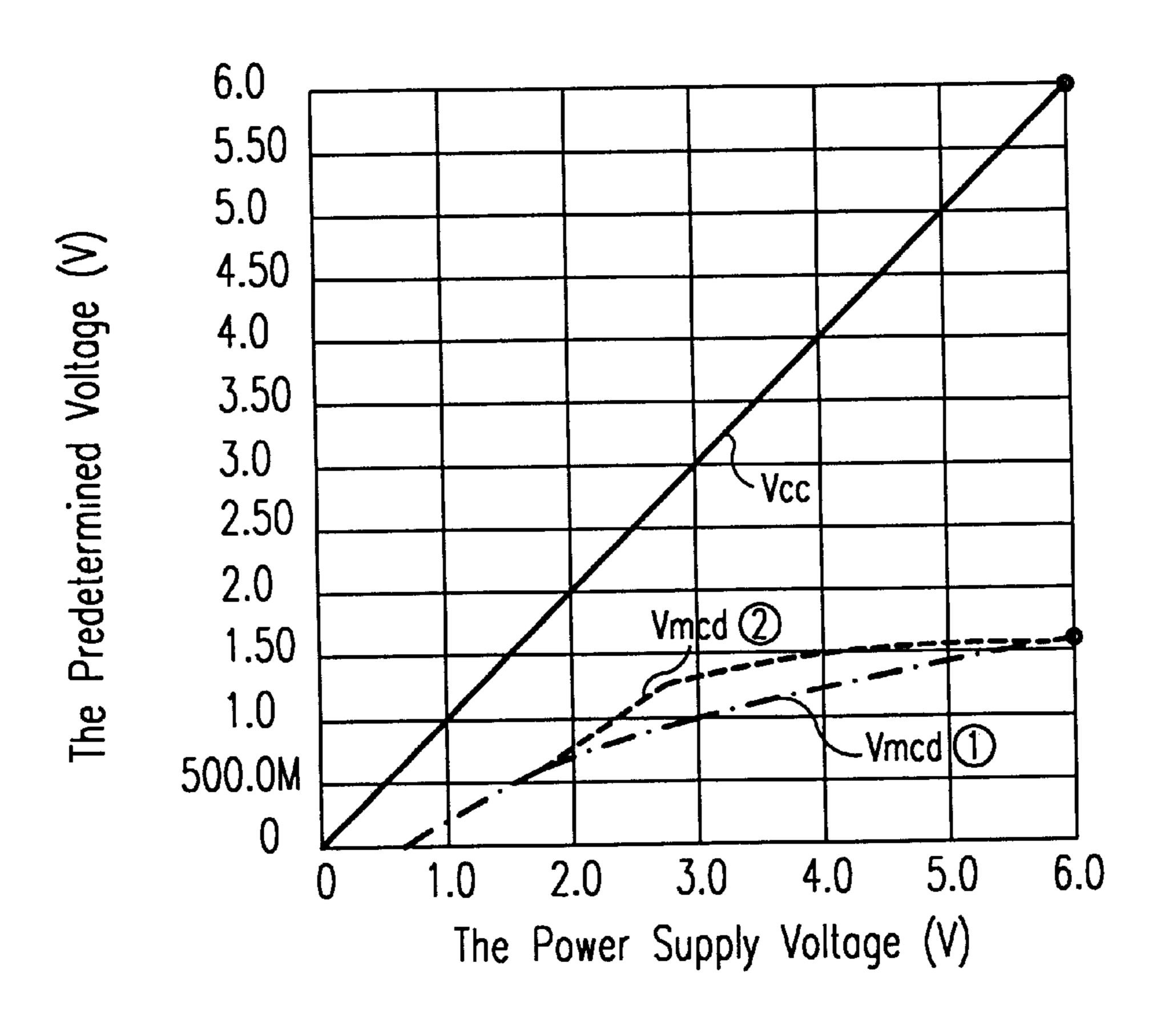
Vmcd (1): Vmcd of the Conventional Constant Voltage Circuit
