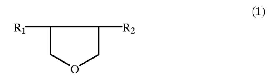
wherein R<sub>1</sub> and R<sub>2</sub> independently represent a hydrogen atom or a straight or branched alkyl group having 1–5 carbon atoms, with a high acid cationic ion exchange resin,
