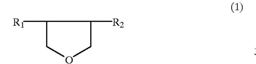
$R_1$  and  $R_2$  independently represent a hydrogen atom or an alkyl group having from 1 to 5 carbon atoms.
