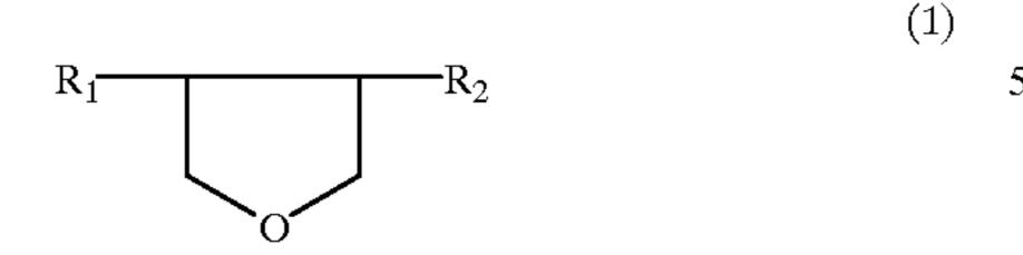
wherein,  $R_1$  and  $R_2$  represent, independently, a hydrogen atom or an alkyl group of 1 to 5 carbon atoms, with mineral acid or a high acid cationic exchanging resin, separating the acidic material from the THF, followed by recovery of the THF by simple distillation and/or rectification to obtain the purified THF.
