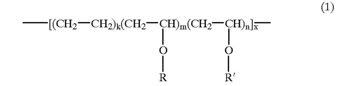
has excellent low-temperature moldability and exhibits an excellent shelf life against softening when stored at high temperatures, and an electrostatic charge developing toner containing the above graft resin as a binder exhibits excellent low-temperature fixing properties, developability and transferability without impairing the shelf life.
