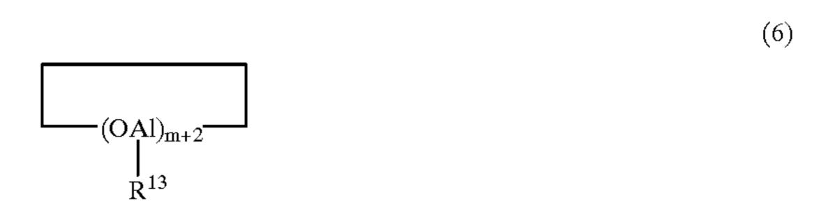
In the above formulae (5) and (6), R<sup>13</sup> is a hydrocarbon group, such as methyl, ethyl, propyl or butyl, wherein preference is given for methyl and ethyl, especially for methyl, and m is an integer of 2 or greater, preferably of 5–40.
