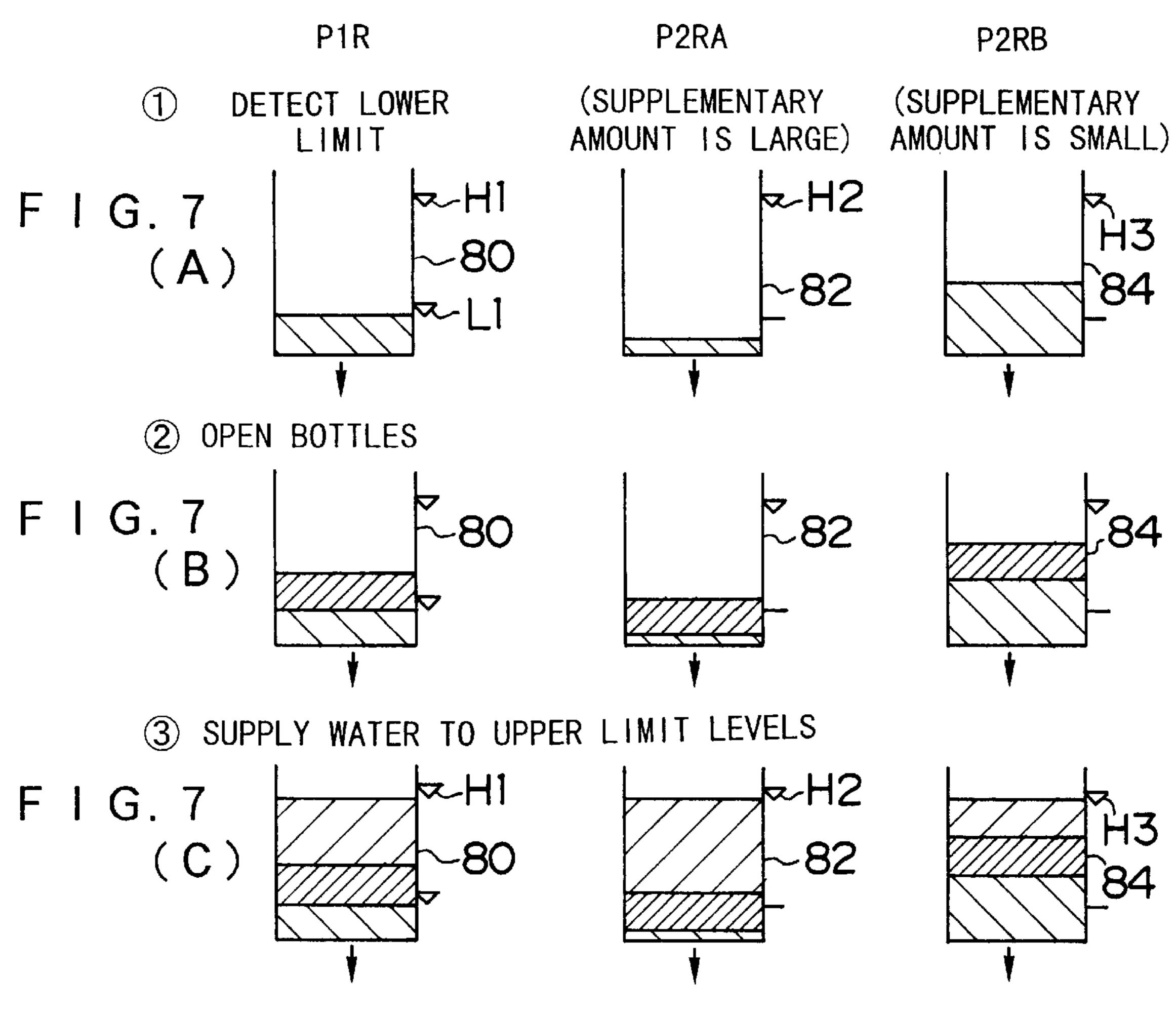
(4) IF SUPPLIED AMOUNT IS LARGER THAN IDEAL VALUE, THIN REPLENISHER IS PRODUCED. IF SUPPLIED AMOUNT IS SMALLER THAN IDEAL VALUE, THICK REPLENISHER IS PRODUCED.
