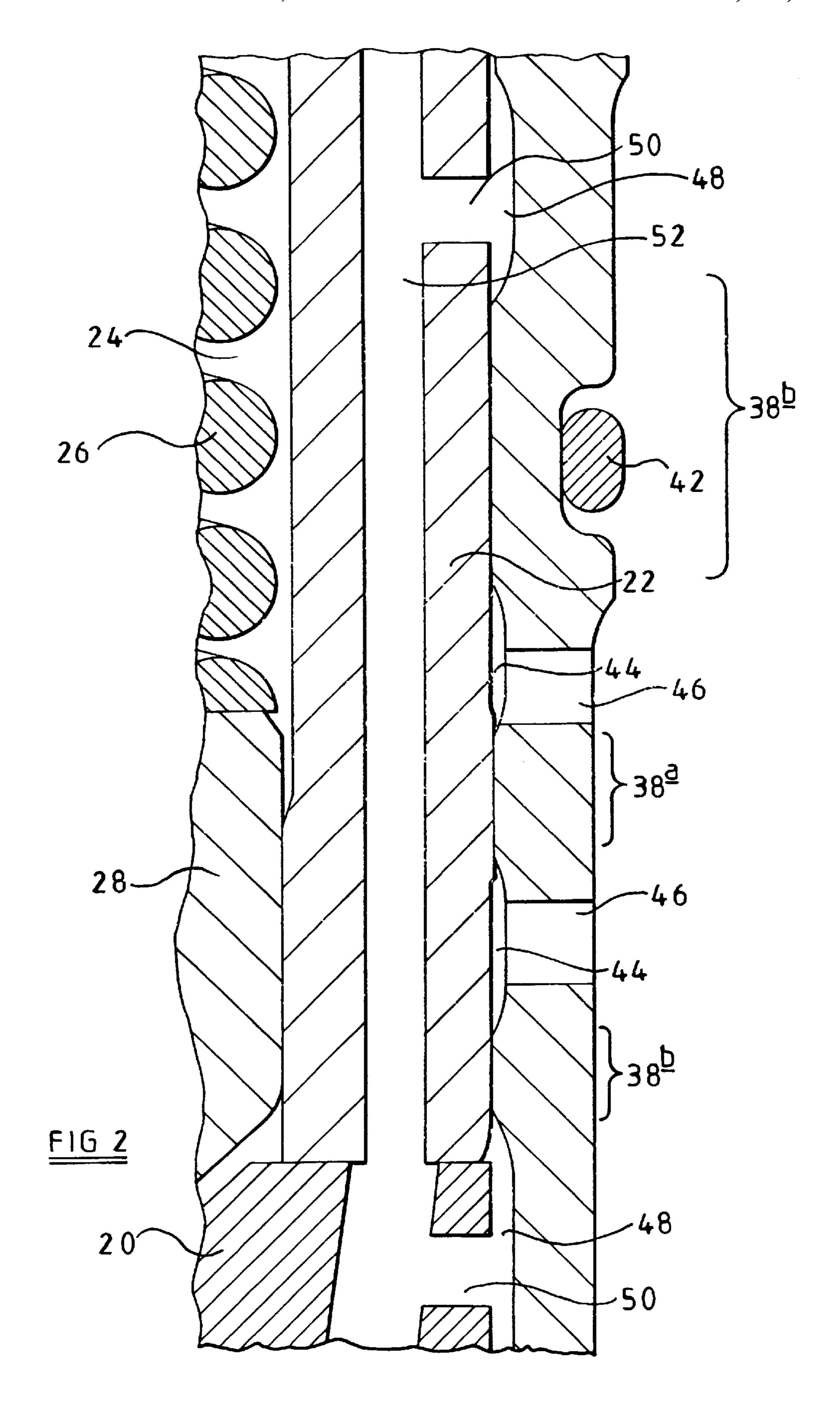
This invention relates to a fuel injector, and in particular to a fuel injector incorporating a filter arrangement for use in removing particulate contaminants from a flow of fuel. 5 The fuel injector may take the form of a pump injector.
