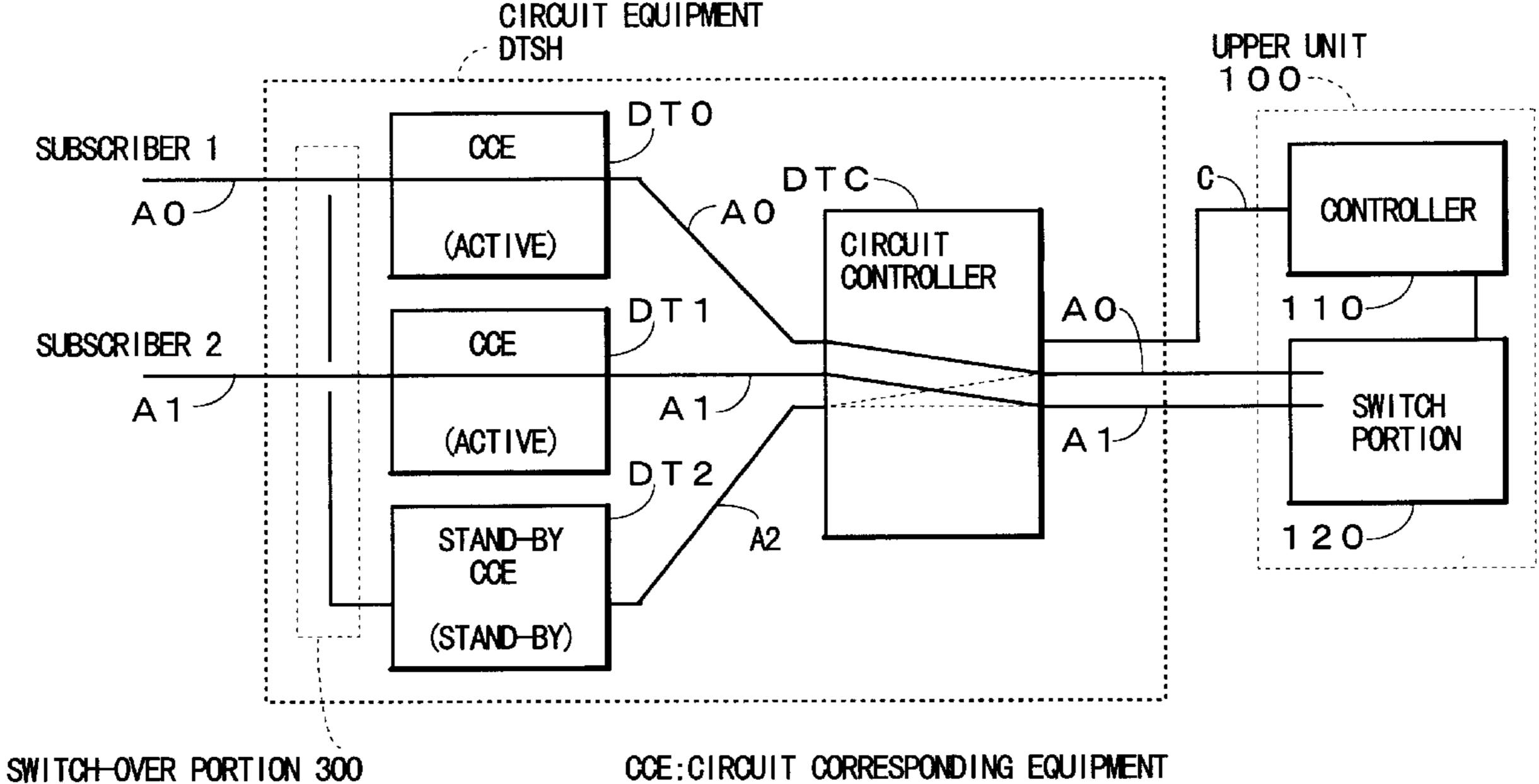
CCE:CIRCUIT CORRESPONDING EQUIPMENT C:CONTROL SIGNAL CIRCUIT AO-A2:MAIN SIGNAL CIRCUIT
