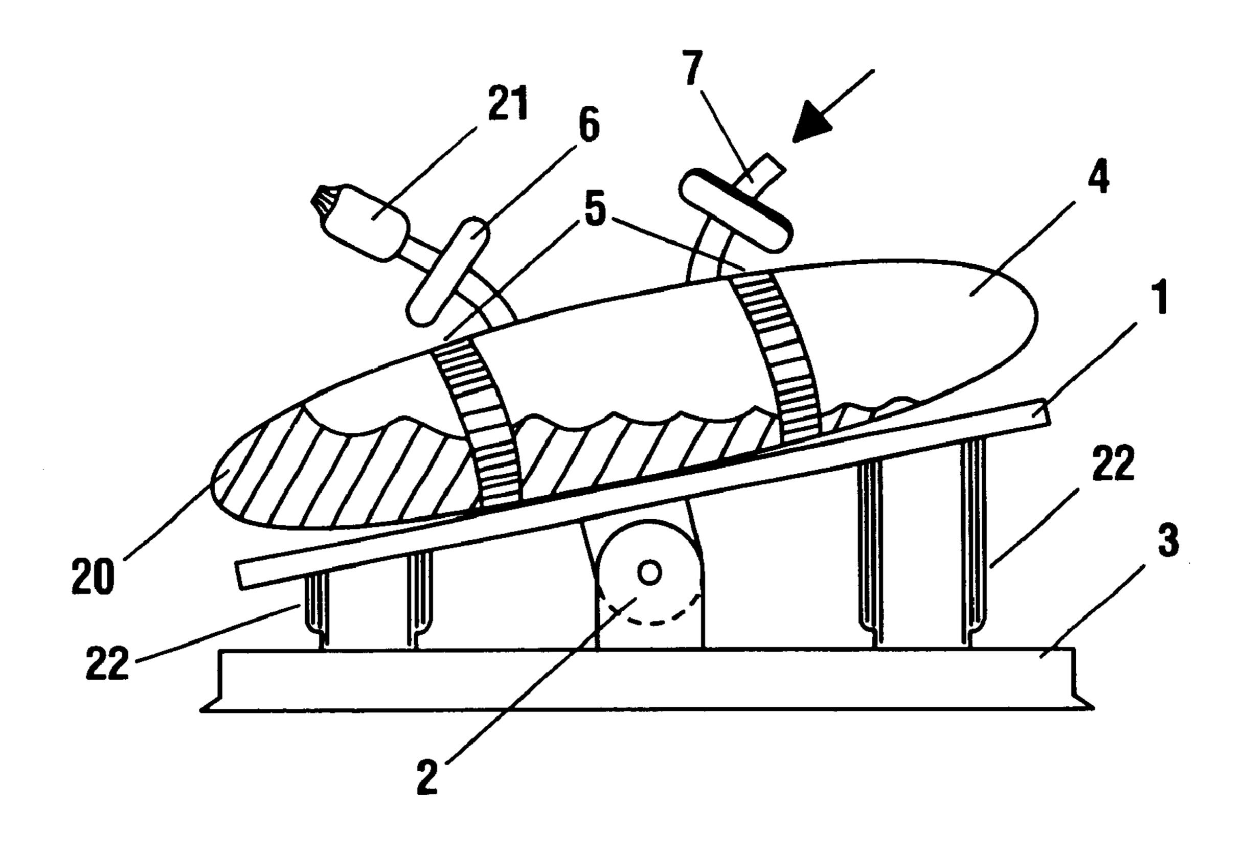
FIG 1. Side view of the apparatus showing bag filled with media and rocking mechanism.
