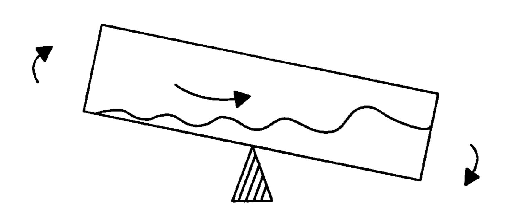
FIG 3. Formation of Waves as a Result of Rocking Motion
