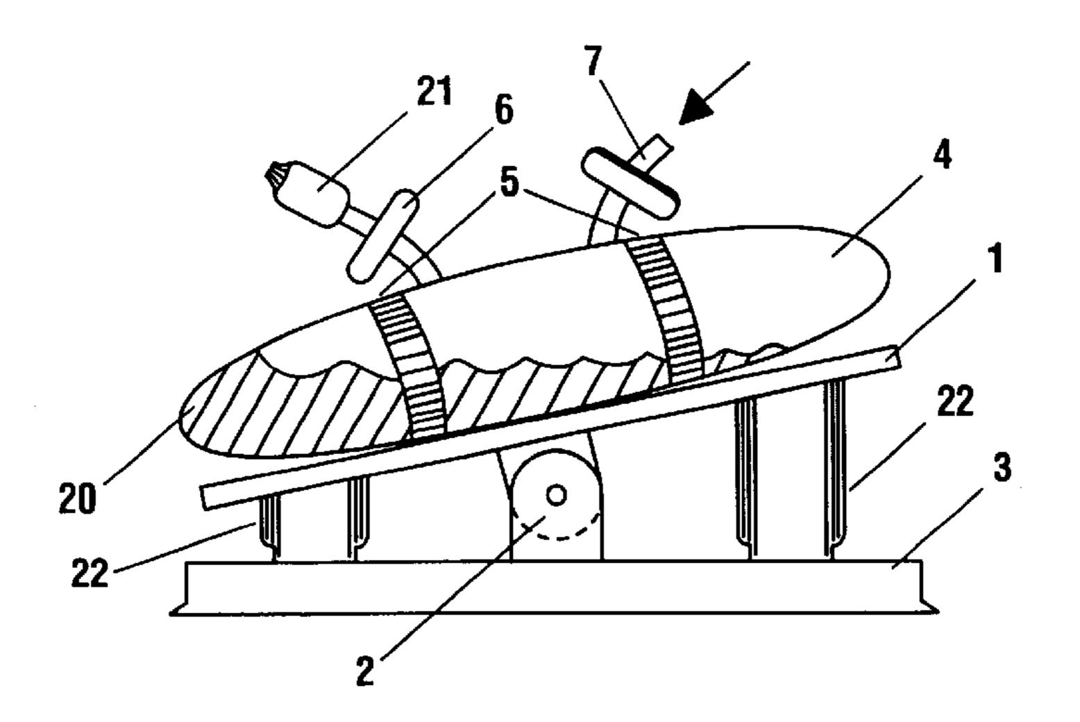
Side view of the apparatus showing bag filled with media and rocking mechanism.
