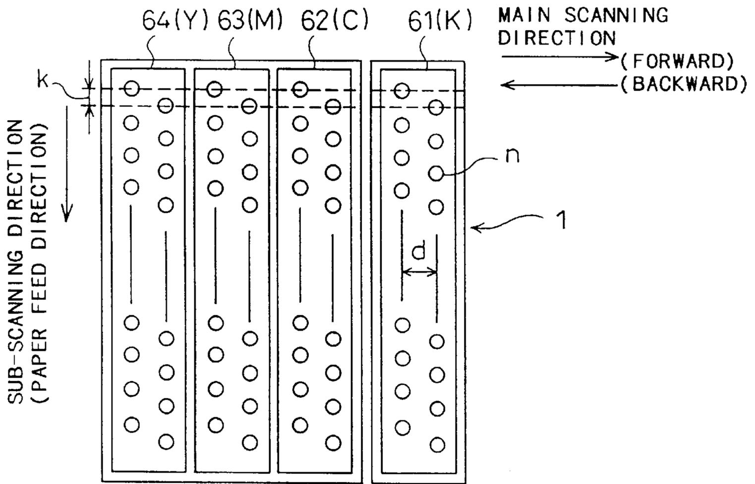
Fig. 3(B) DOTS FORMED BY ONE NOZZLE ARRAY
