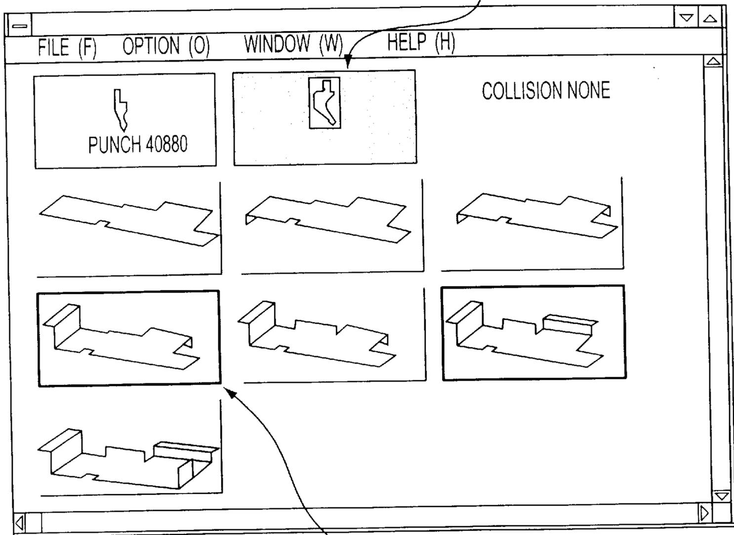
IN CASE OF USE A SECOND PUNCH, A SECTION WILL BE HIGHLIGHTED WITH DIFFERENT COLOR.
