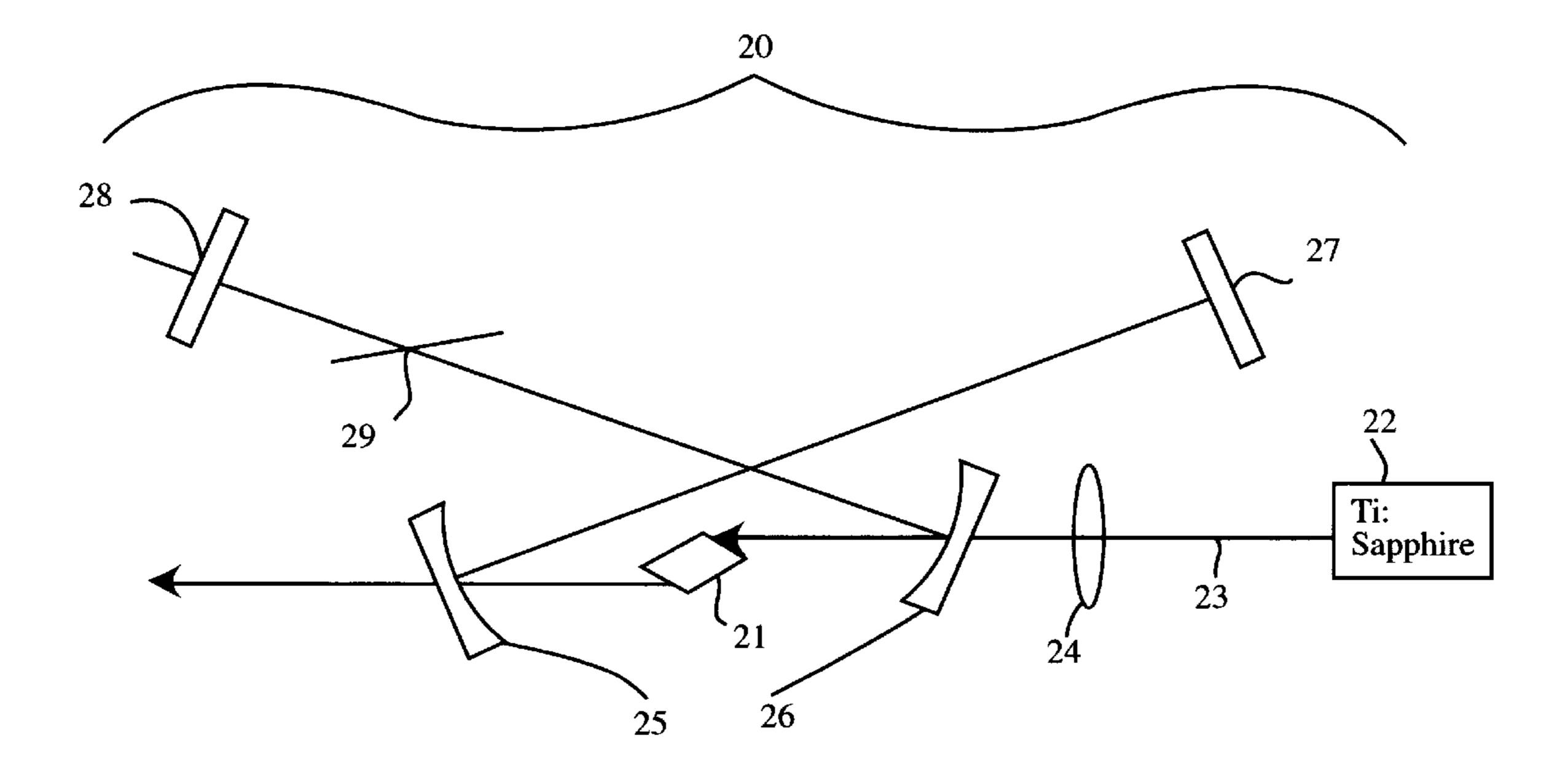
X-cavity schematic; f = 12.5cm, 2% O.C., 10cm ROC curved mirrors, 10% YB dopant, 10 mm long Brewster/Brewster cut crystal.
