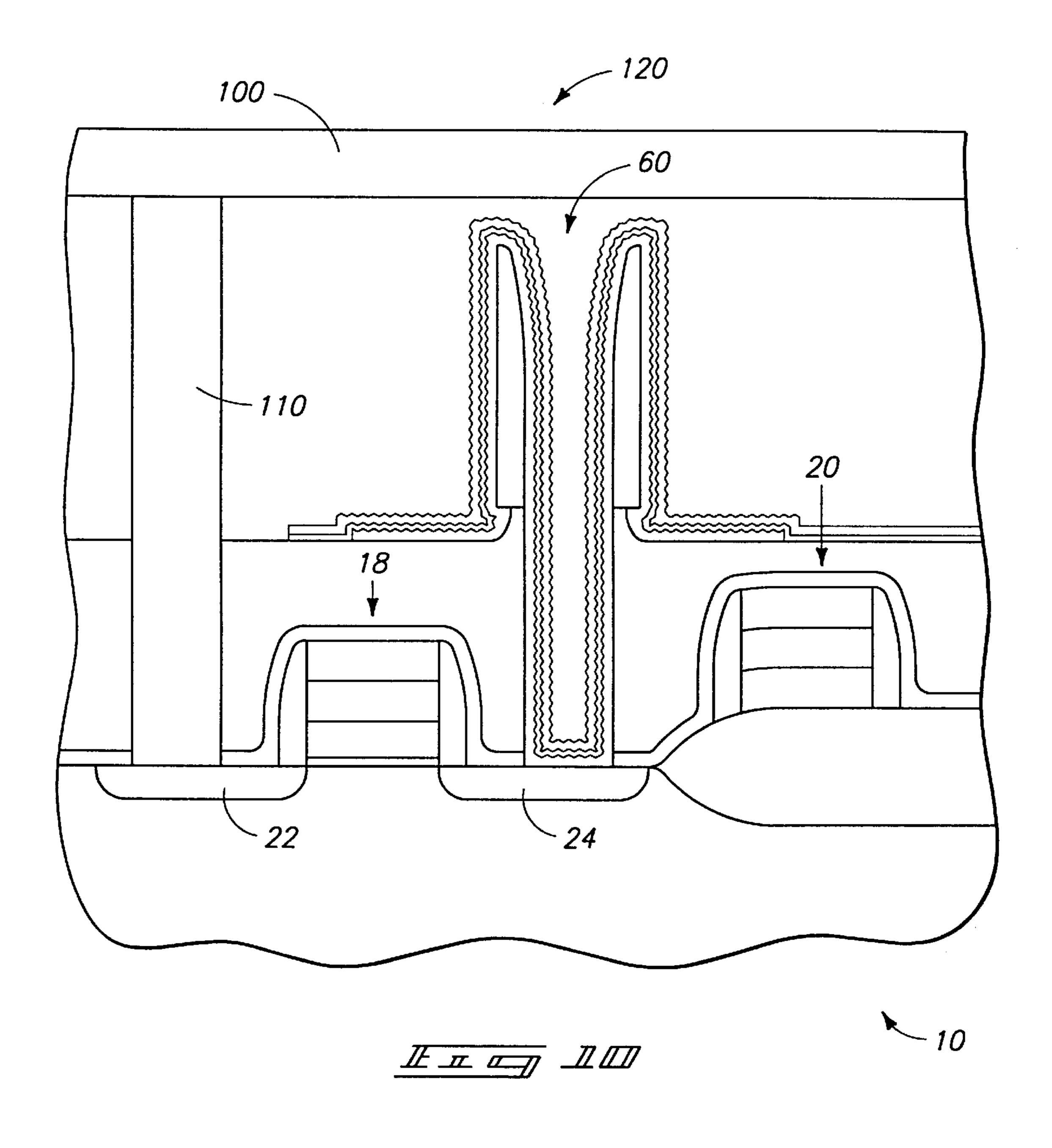
CAPACITOR STRUCTURES, DRAM CELL STRUCTURES, METHODS OF FORMING CAPACITORS, METHODS OF FORMING DRAM CELLS, AND INTEGRATED CIRCUITS INCORPORATING CAPACITOR STRUCTURES AND DRAM CELL STRUCTURES
