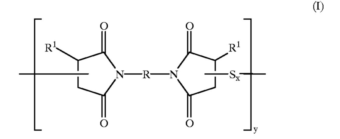
wherein R is selected from the group consisting of phenylene and xylylene; R<sup>1</sup> is selected from the group consisting hydrogen and alkyls having from 1 to 18 carbon atoms; x is an integer of from 2 to 8 and y is an integer of from 2 to 10.
