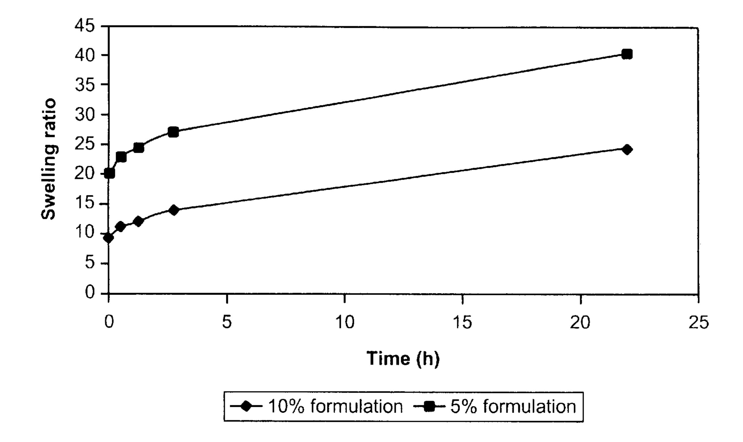
Swelling ratio = (Total weight of hydrogel) / (Weight of prepolymer)
