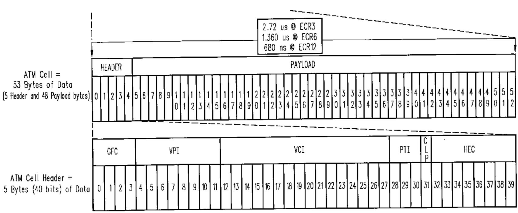
ATM Cell Header Bit Definitions Bit 1 Delay control bit
