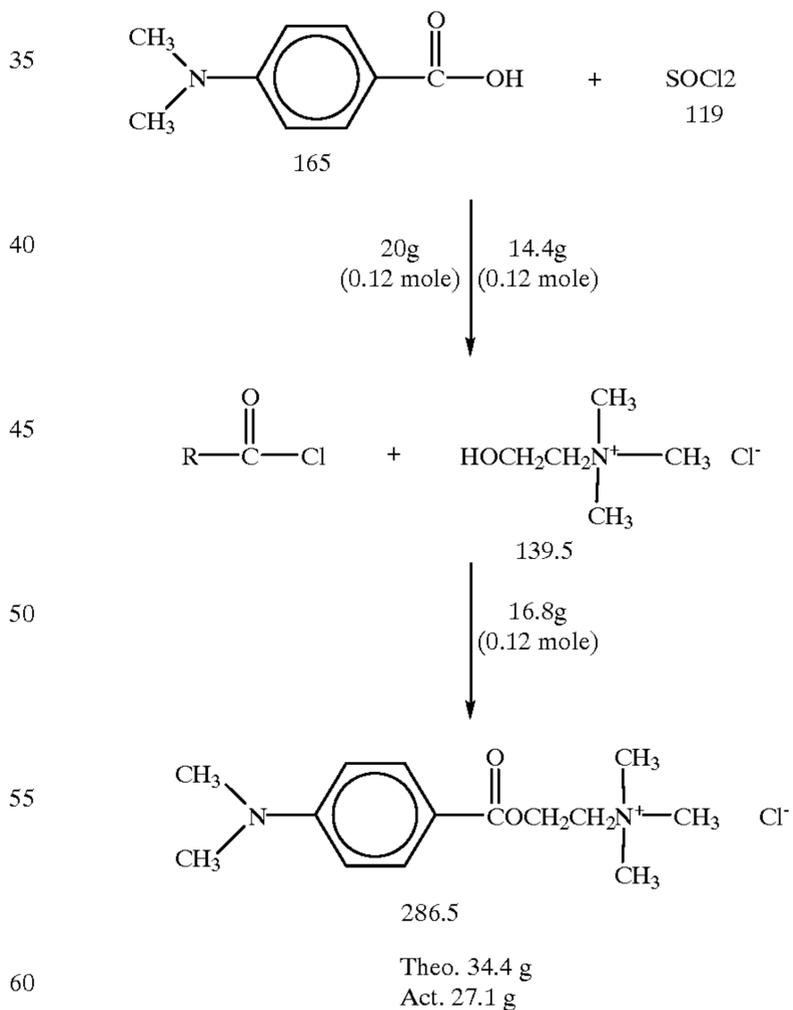
Into a 3 necked 500 ml. round bottomed flask fitted with magnetic stirrer and condenser was added 20 g (0.12 moles) dimethyl amino benzoic acid (Aldrich) and 100 ml. of toluene. The Dean-Stark adapter was fitted and 80 ml. of toluene (Aldrich anhydrous grade) 14.4 g (0.12 mole) thio-
