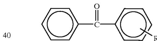
wherein R represents any substituents which permit the benzophenone to function as a colorant stabilizer.
