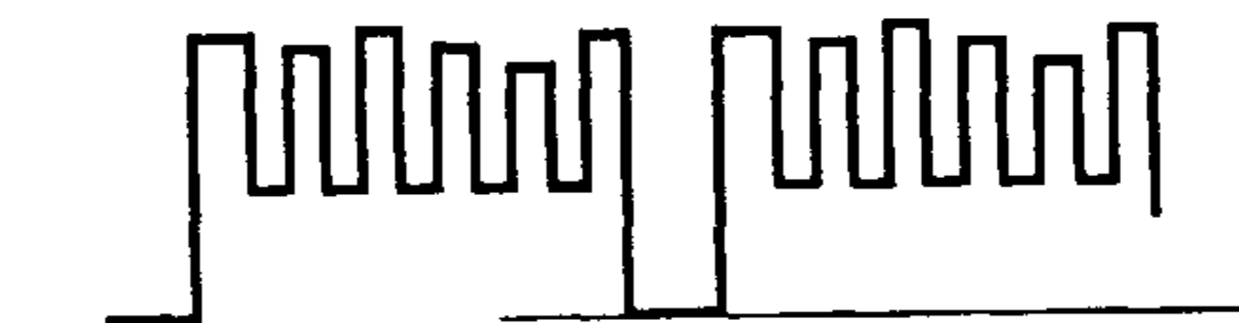
FIG. 11(f) DARK CLAMPING OUTPUT (WHEN LEVELS AT BLACK PORTIONS ARE HIGH IN DOCUMENT MODE)
