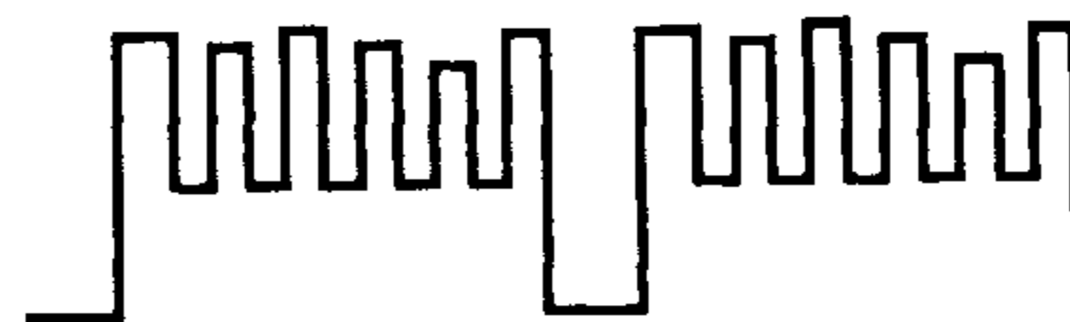
FIG. 11(b) OUTPUT FROM PRE-PROCESSING CIRCUIT (WHEN LEVELS AT BLACK PORTIONS ARE HIGH IN DOCUMENT MODE)
