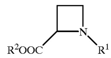
wherein R<sup>1</sup> has the same meaning as defined above and R<sup>2</sup> denotes an alkyl group, an aralkyl group or an allyl group, with an enzyme capable of selectively hydrolyzing a stereoisomer based on the carbon atom of the 2-position of the azetidine ring.
