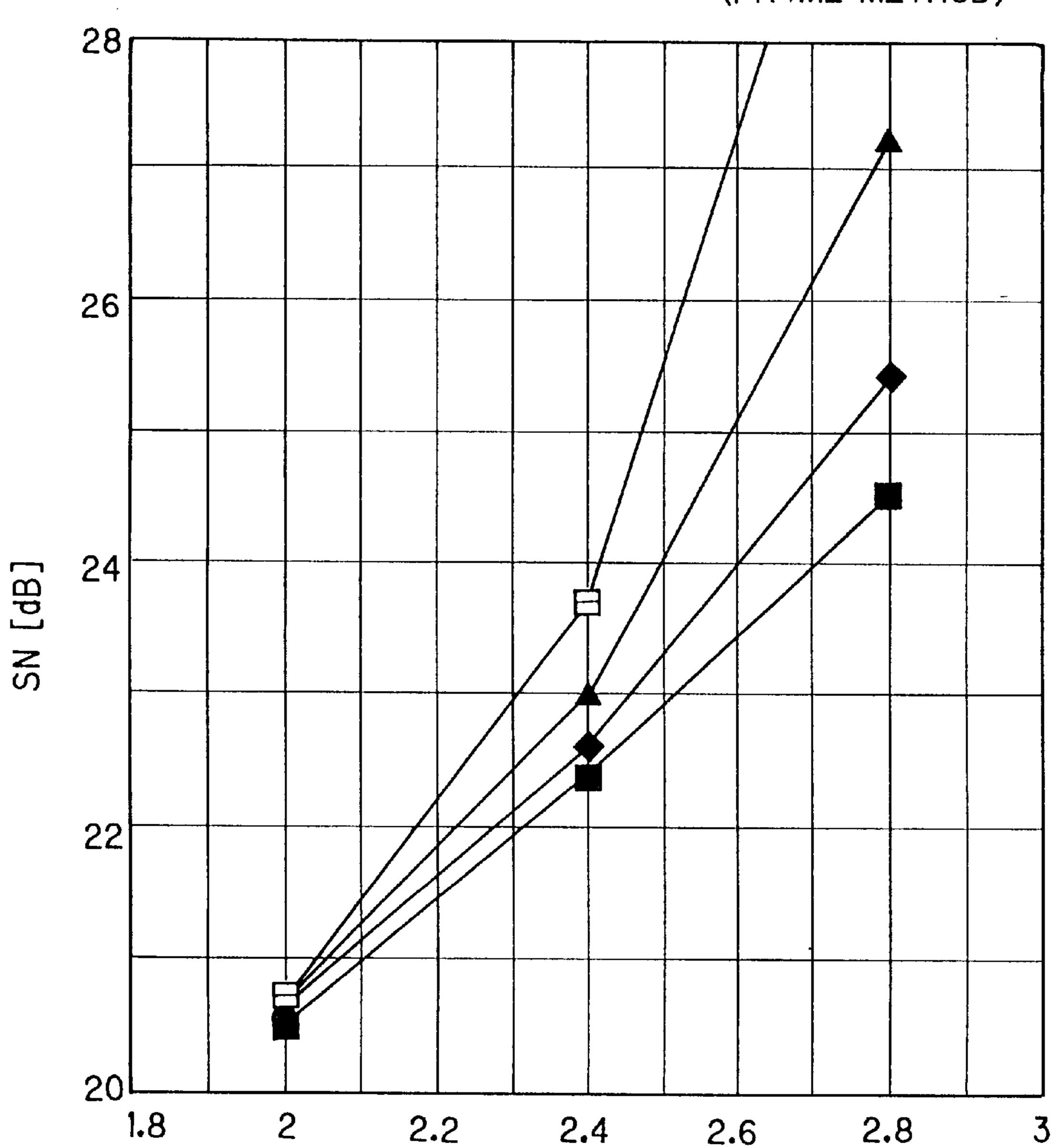
K=PW50(HALF PEAK WIDTH)/BI(MINIMUM BIT INTERVAL)
