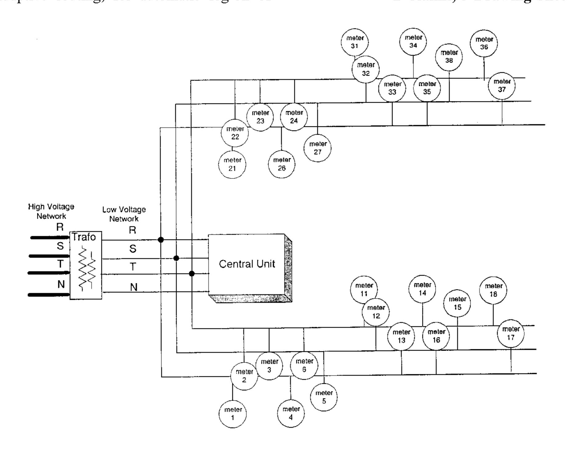
Figure 1 - typical PLC network
